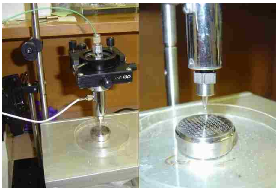
Figure 2-8. A photograph of the piezoelectric-actuated droplet generator mounted in XYZ stage with droplet ejection onto a commercial MALDI target.
