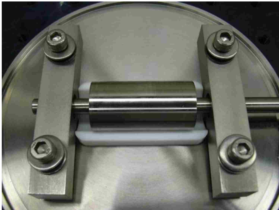
Figure 7-1. Cylinder inlet interface.
