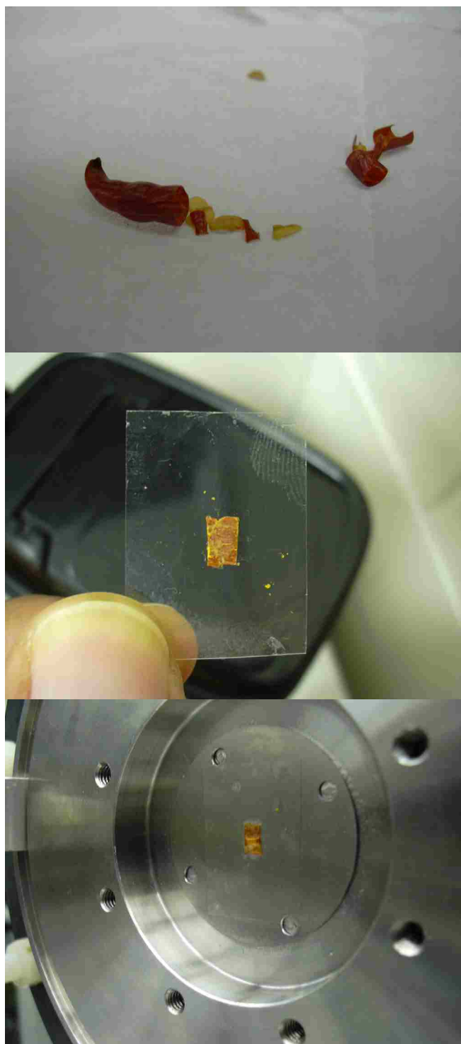
Figure 6-1. Preparation of dehydrated chili pepper tissue for direct desorption/ionization analysis. Tissue sections were spotted with matrix and affixed to adhesive tape with the membrane side exposed. The tape was then brought into contact with the direct desorption interface with the tissue section directly over the interface orifice, creating a vacuum seal.
