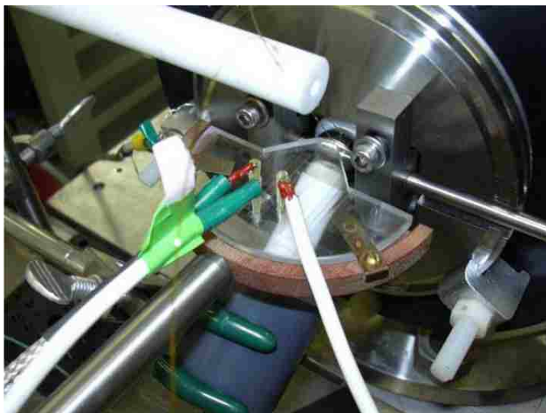
Figure 3-5. A photograph of on-line microfluidic chip detection with ball inlet MALDI-MS.
