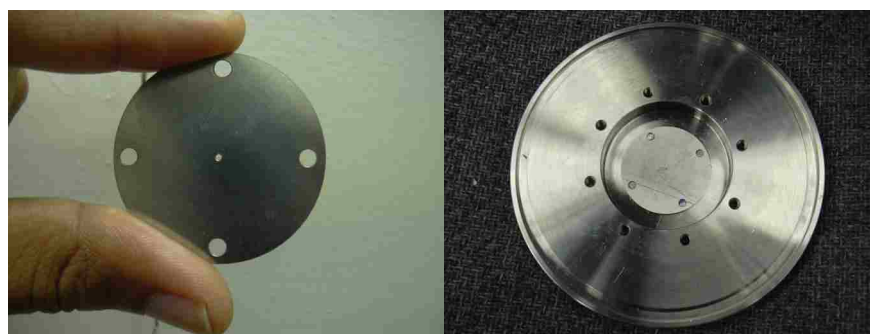
Figure 6-3. Direct desorption/ionization interface. The plate (left) contains a 1 mm orifice for sample irradiation with laser light and sits in the center of an ISO 100 flange (right).
