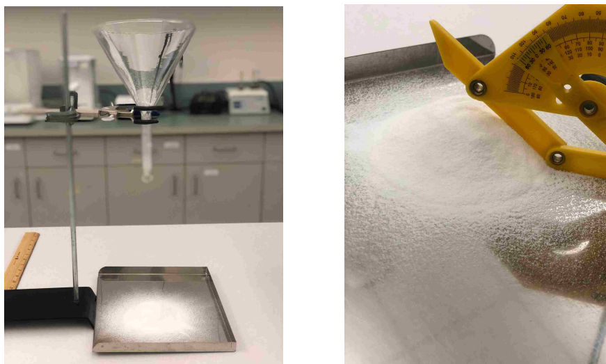
Figure 10. Measurement of the powder's angle of repose using a goniometer angle finder, miter gauge arm, measuring ruler protractor.
