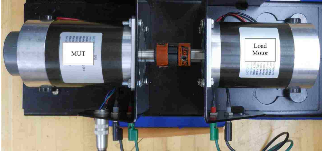
Figure 3.3 MUT axially coupled to load motor (seen in laboratory)
