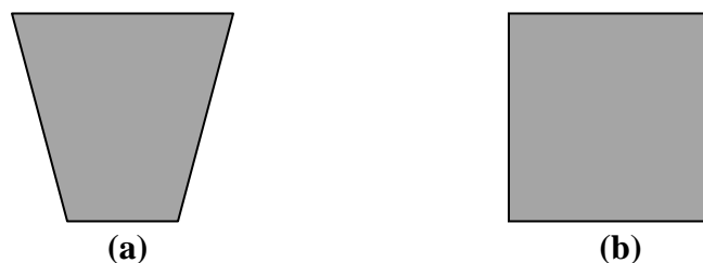
Fig. 3.6. (a) Trapezoidal PM pole, (b) Rectangular PM pole
