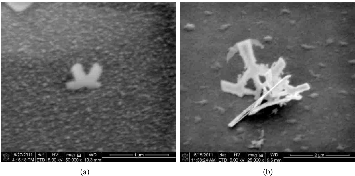
Figure 6.1. SEM images at different stages of hexagonal diamond formation. (a) early stage of hexagonal diamond platelet growth, (b) early stage of graphene layer(s) formation, (c) connection of radial spokes with graphene layer(s), (d) beginning stage of spaces filling up, (e) more filled up stage and (f) almost filled up hexagonal diamond platelet. The scale bar shown in a, d and e is 1 μm long and that in b, c and f is 2 μm long.
