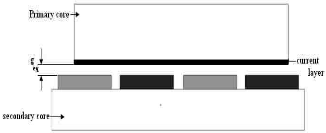
Figure 3.5 Schematic representation of unslotted primary core
