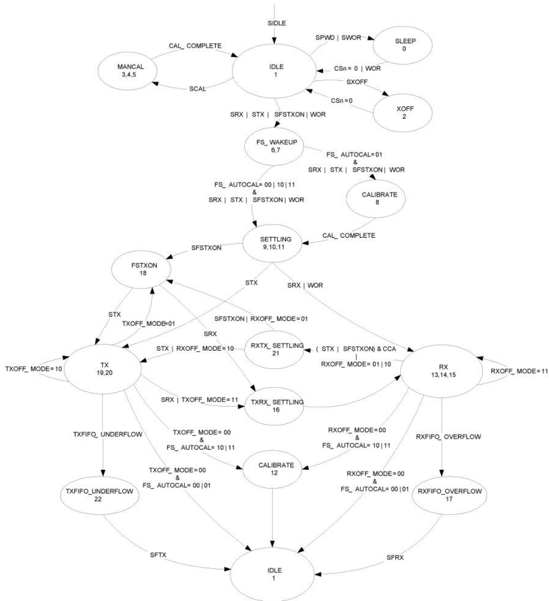
Figure 13. Radio Mode Control State Diagram
