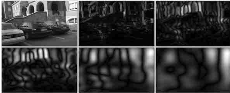
Figure 17: Second order image derivative in x-direction.
