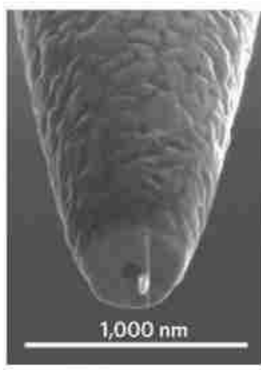
FIGURE 1.2. An aperture-based probe consisting of a metal protrusion deposited adjacent to an NSOM aperture.
