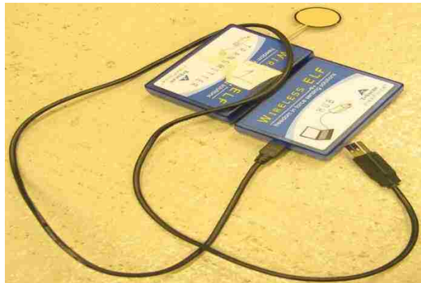
Figure 5: Wireless ELF system (Force sensors, Transmitter and Receiver) is used to measure the static forces.
