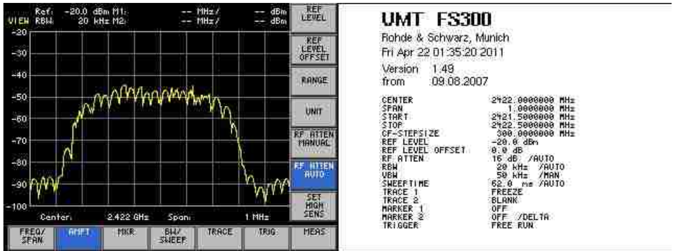
Figure 3.4: PSD of DBPSK modulated waveform on Spectrum Analyzer
