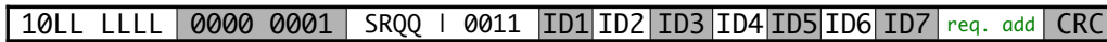
FIGURE 4.16: Packet of sub-type b0011. This packet is created by a module interested in getting initialized. The packet contains the 7 byte ID of the module, which is further broken into a 6 - byte ID segment and a 1-byte family type. The module can request for a preferred address to be allocated using the optional (marked green) “req. add” field. The parameter S denotes address type: 0 - if only static address is possible & 1 - if both static and dynamic address are possible; parameter R denotes address memory: 1 - if it can remember address after brownout reset & 0 - otherwise; parameter QQ denotes additional addresses being requested for other modules limited to a maximum of four. The length of the packet is dependent on the presence of the optional “req. add” field.
