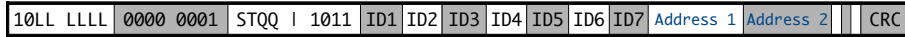
FIGURE 4.25: Packet of sub-type b1011. The packet created by a module on accepting the assigned slave address. The packet is similar to one in Figure 4.23, except for the sub-type field and the CRC.
