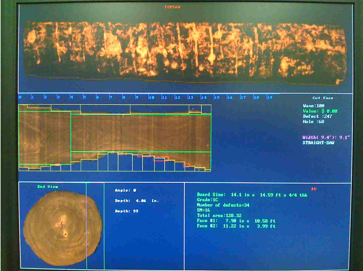
FIGURE 5.9: The image of cutting 3D virtual log.
