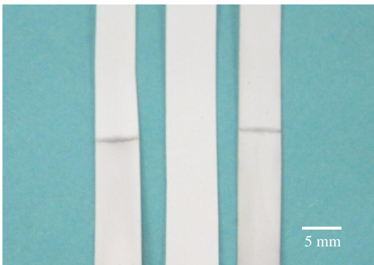
Figure 4.7 Non-specific adsorption on the nitrocellulose membrane (i) carbon nanotubes partially coated with PVP bound to Protein A by non-specific adsorption which must be addressed to avoid false signal (ii) almost no carbon nanotubes at the capture line showing that the surface of carbon nanotubes were completely covered eliminating non-specific adsorption after the application of crosslinking agent, EDC, and Sulfo-NHS, and (iii) binding between the MWCNT-IgG conjugate and immobilized Protein A.
