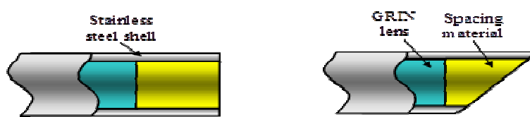
Figure 3.1.6. Cross section view of (a) blunt and (b) sharp endoscopic probes. (Feldman et al)
