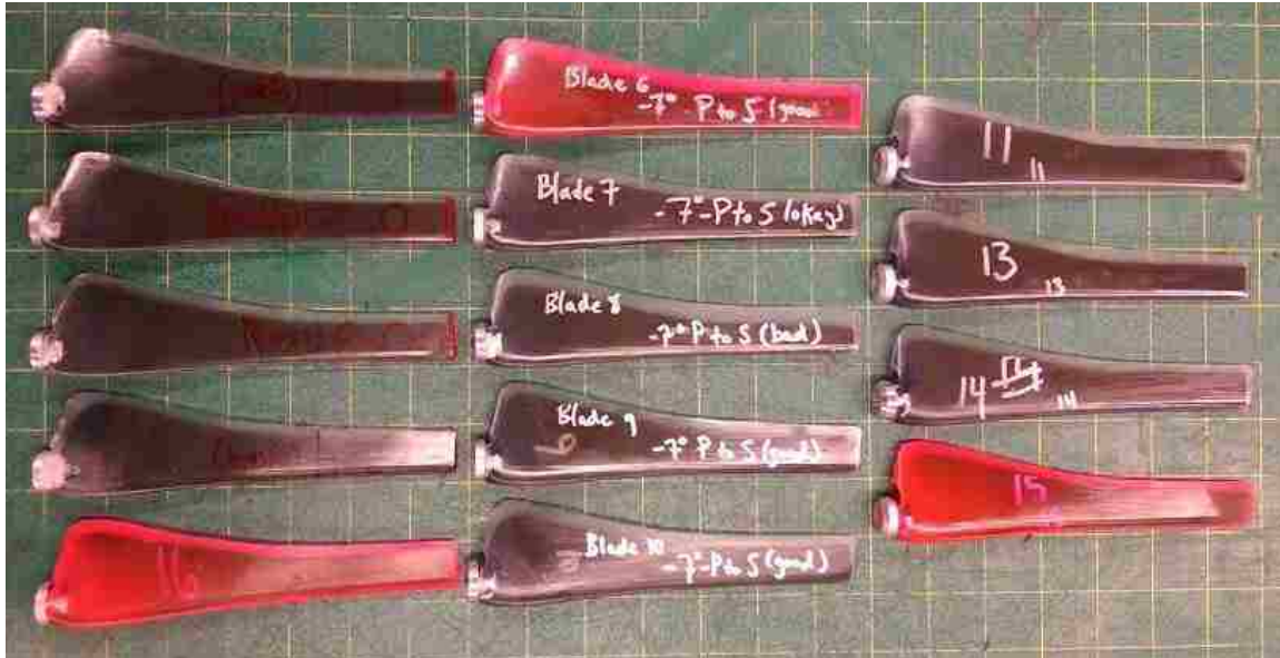
Figure 6.7: Composite blade sets; semi-flexible urethane over twisted composite spar.
