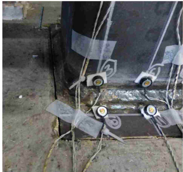
Figure 6.5.2.2.b: Close up of Specimen 4-0-0.92 at P=60kips
