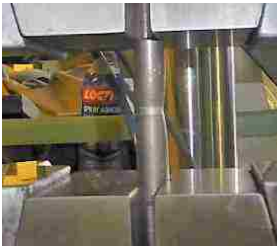
Figure 6.3.2.5: Stud shank test (necking and fracture photos)
