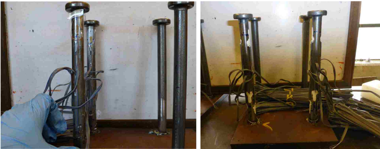
Figure 6.4.2.1: Installed Strain gauges (before and after M-Coat application)
