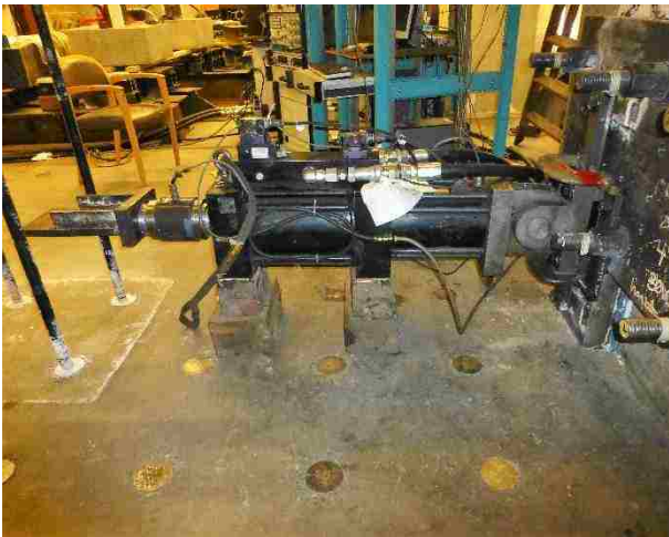
Figure 6.4.1.4.a: Actuator sitting on timber pieces
