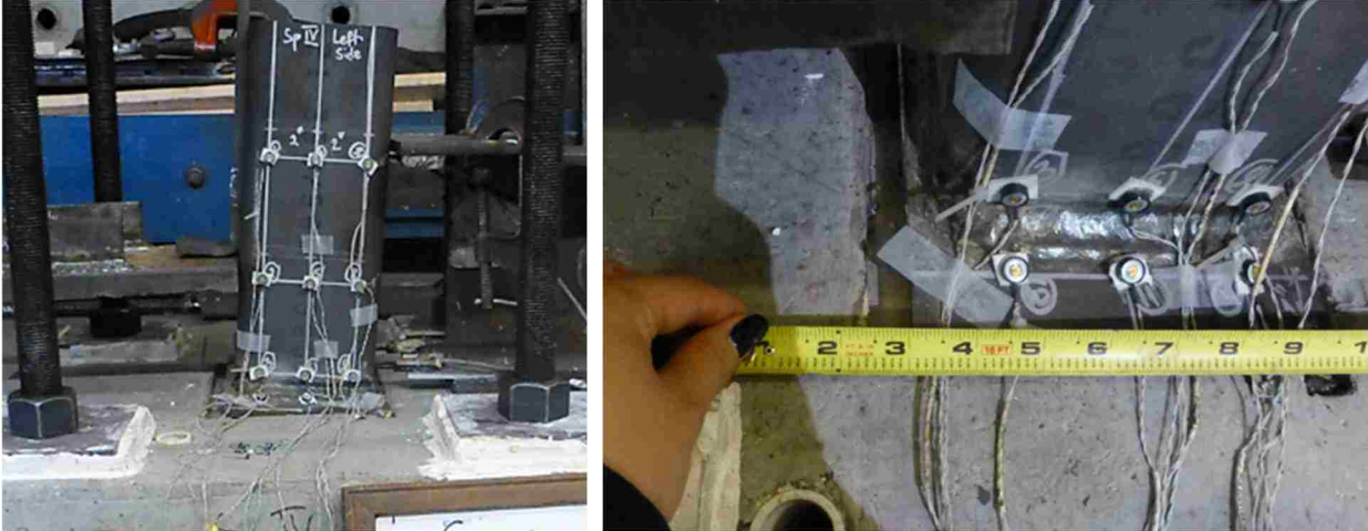
Figure 6.5.2.4: Specimen 4-0-0.92 at failure
