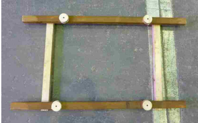
Figure 6.2.5.2: Frame with plugs for the steel pipes
