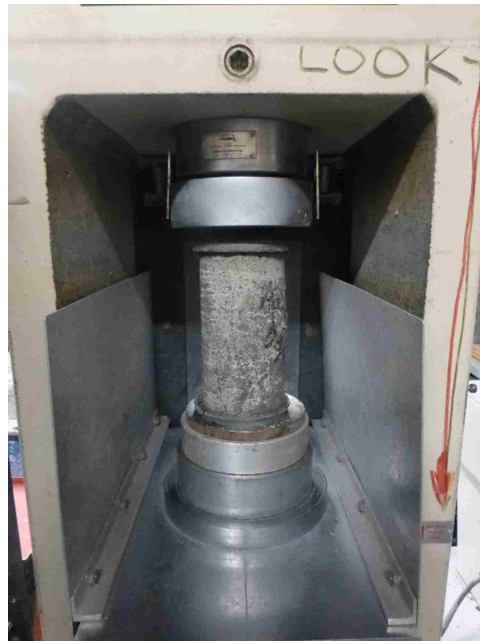
Figure 6.3.1.2: Compressive strength test set up
