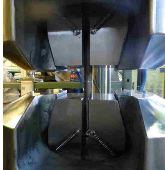
Figure 6.3.2.4.a: Test set up for tensile strength of studs (close-ups)
