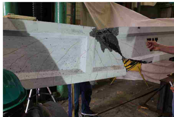
Figure 1.1.1: Diagonal web shear failure in a prestressed concrete beam (UW Big Beam Competition team media, 2016)
