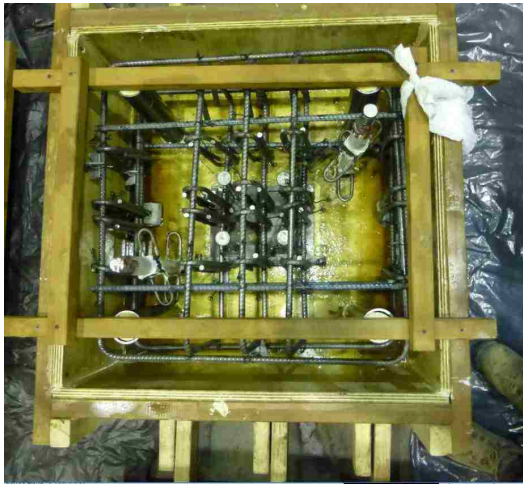
Figure 6.2.5.5: Strain gauge wires protected for casting process
