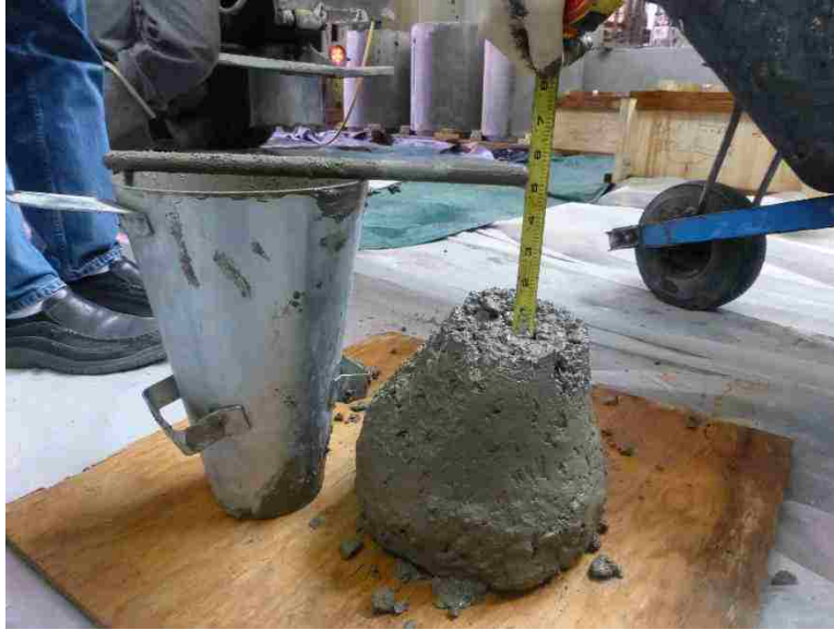
Figure 6.3.1.1: Slump test result
