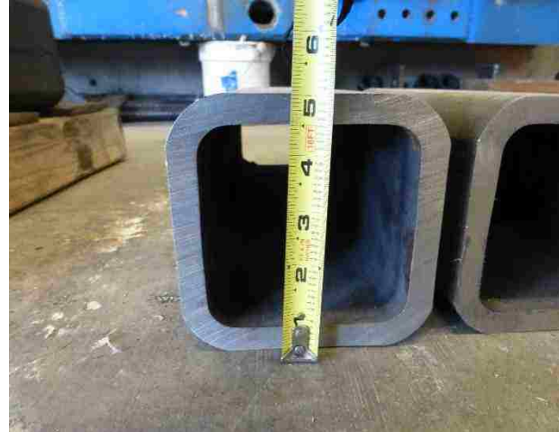
Figure 6.4.1.2.b: 5"x5" HSS tube for 2-stud specimen
