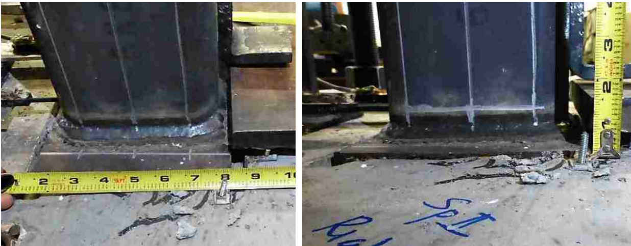
Figure 6.5.4.4: Photographs of slip and crack width after failure (Specimen 2-2-0.25)
