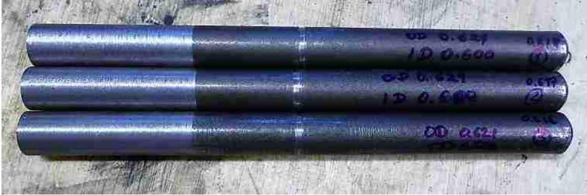
Figure 6.3.2.3: Machined stud shanks for tensile tests
