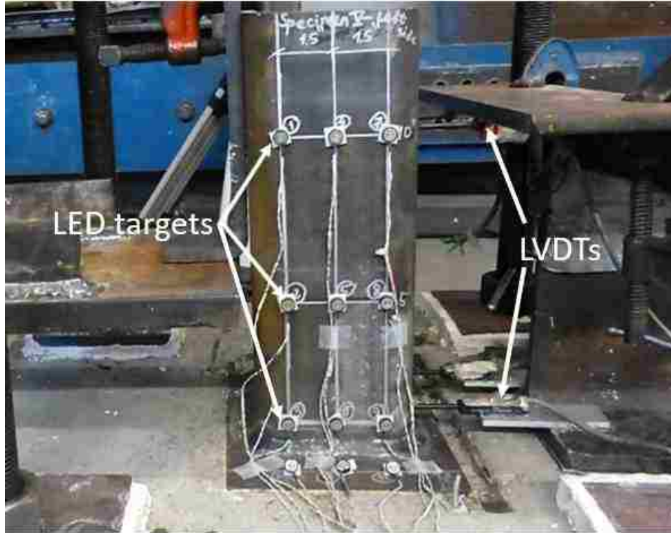
Figure 6.4.2.3: Close up of displacement sensors and the tip of actuator gizmo
