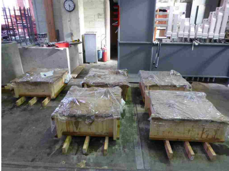
Figure 6.2.6.2: Moisture curing set up for test specimens
