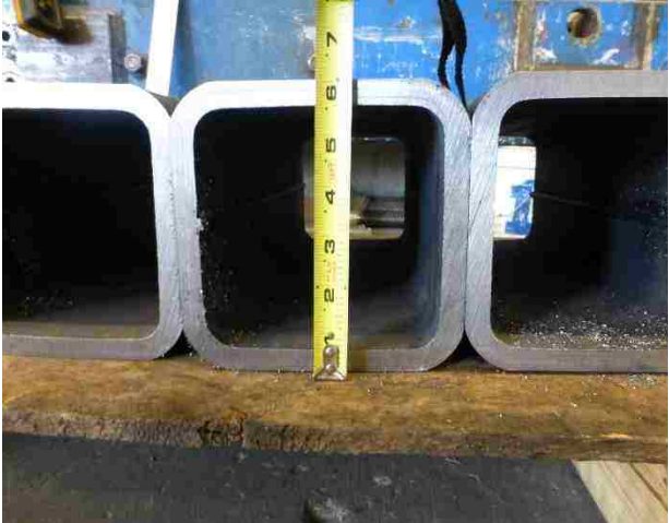
Figure 6.4.1.2.a: 6"x6 HSS tubes for 4-stud specimens
