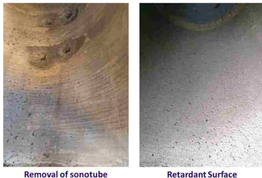
Figure 7-12. Comparison of surface roughness after removal of sonotube, with and without retardant
