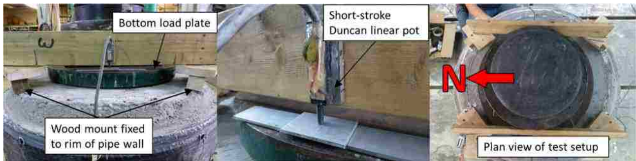
Figure 4-12. Linear Potentiometers used to measure vertical displacement of plug
