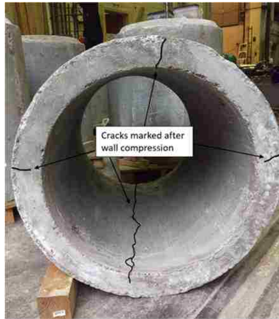
Figure 4-9. Longitudinal cracks - Specimen ep24-cr
