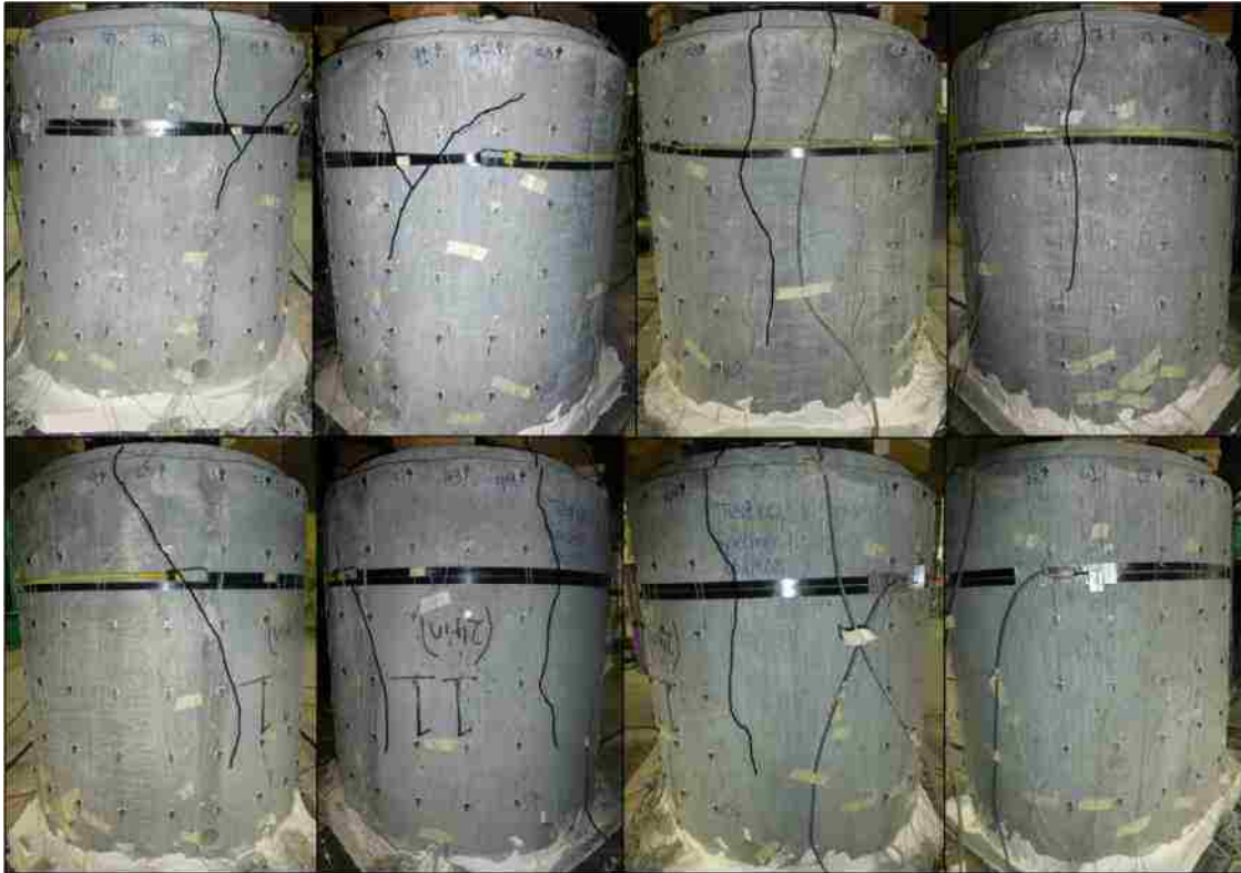
Figure 5-6. Crack formation at peak load for Test ep24-2 (L-R: N-NW-W-SW; S-SE-E-NE)
