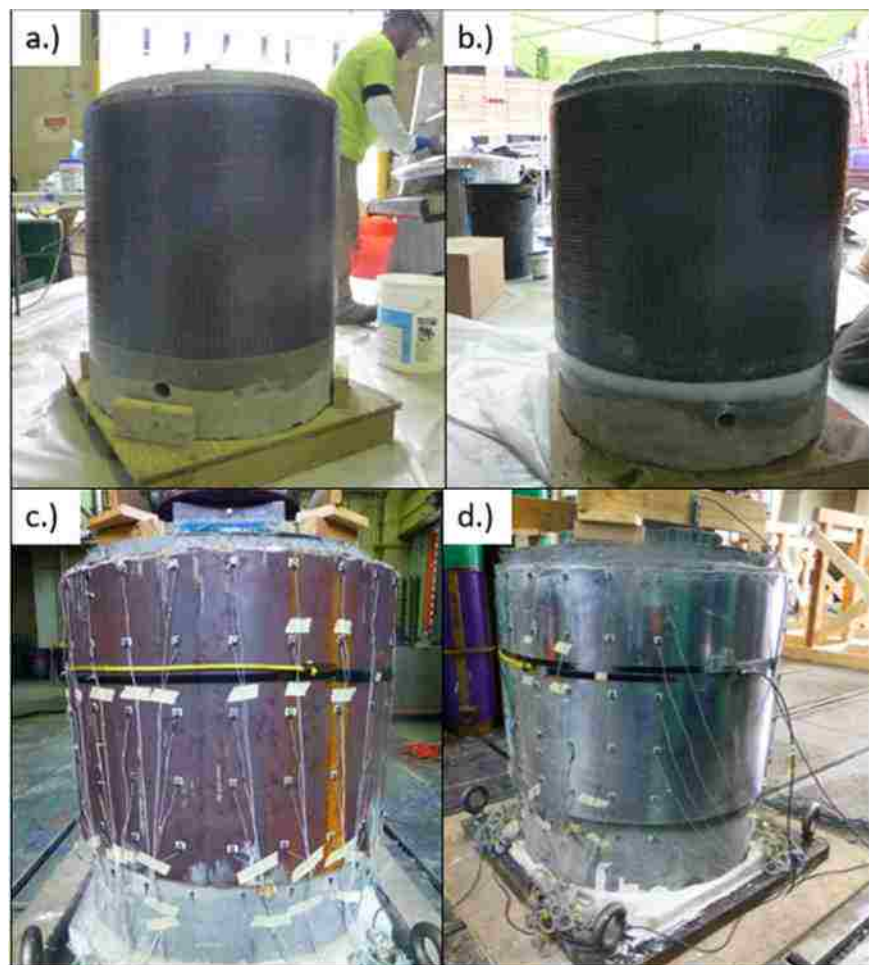
Figure 4-10. Jacketed Specimens - a.) 1-layer CFRP (ep24f1-1); b.) 6-layer CFRP (ep24f6-1); c.) ¼”-thick steel jacket (ep24s4-1); d.) 1/16”-thin steel jacket (ep24s1-1)
