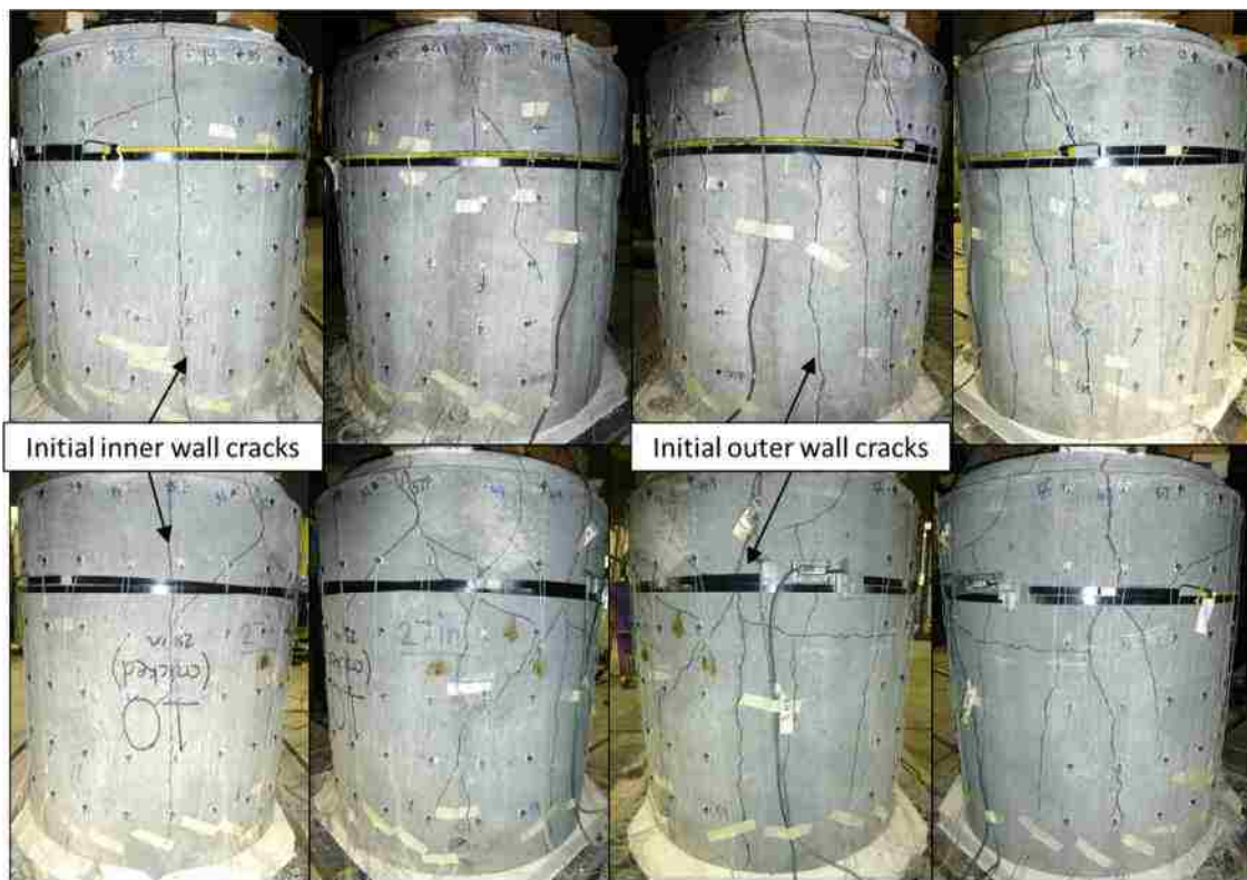
Figure 5-13. Crack Formation at Peak Load for Test 6-ep24-cr (L-R: N-NW-W-SW; S-SE-E-NE)
