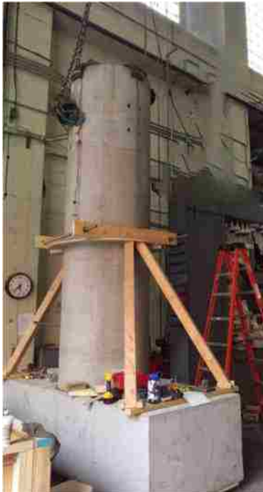
Figure 7-19. Column braced on top of cap beam
