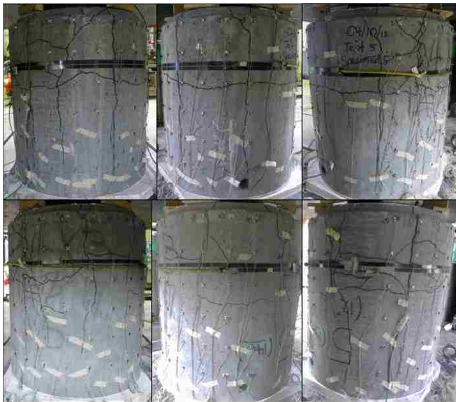
Figure 5-12. Crack formation at end of testing for Test ep14-1 (L-R: N-NW-SW; S-SE-NE)
