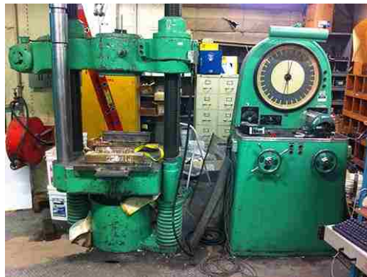
Appendix Figure H.2 300-kip Baldwin testing machine.
