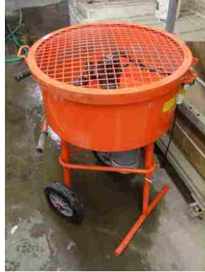
Appendix Figure H.1. Pan mixer used to mix UHPC.
