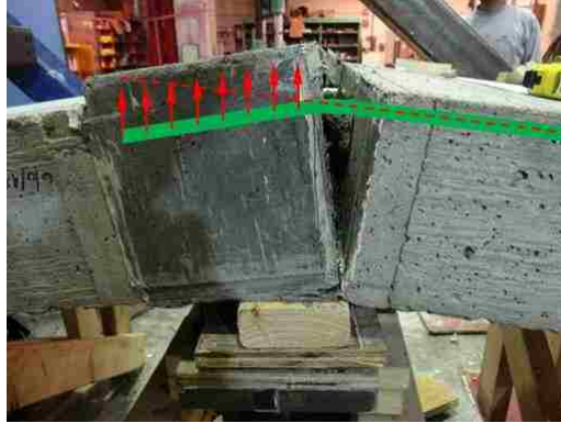
Figure 7.8. Upward force distribution from bent reinforcement.
