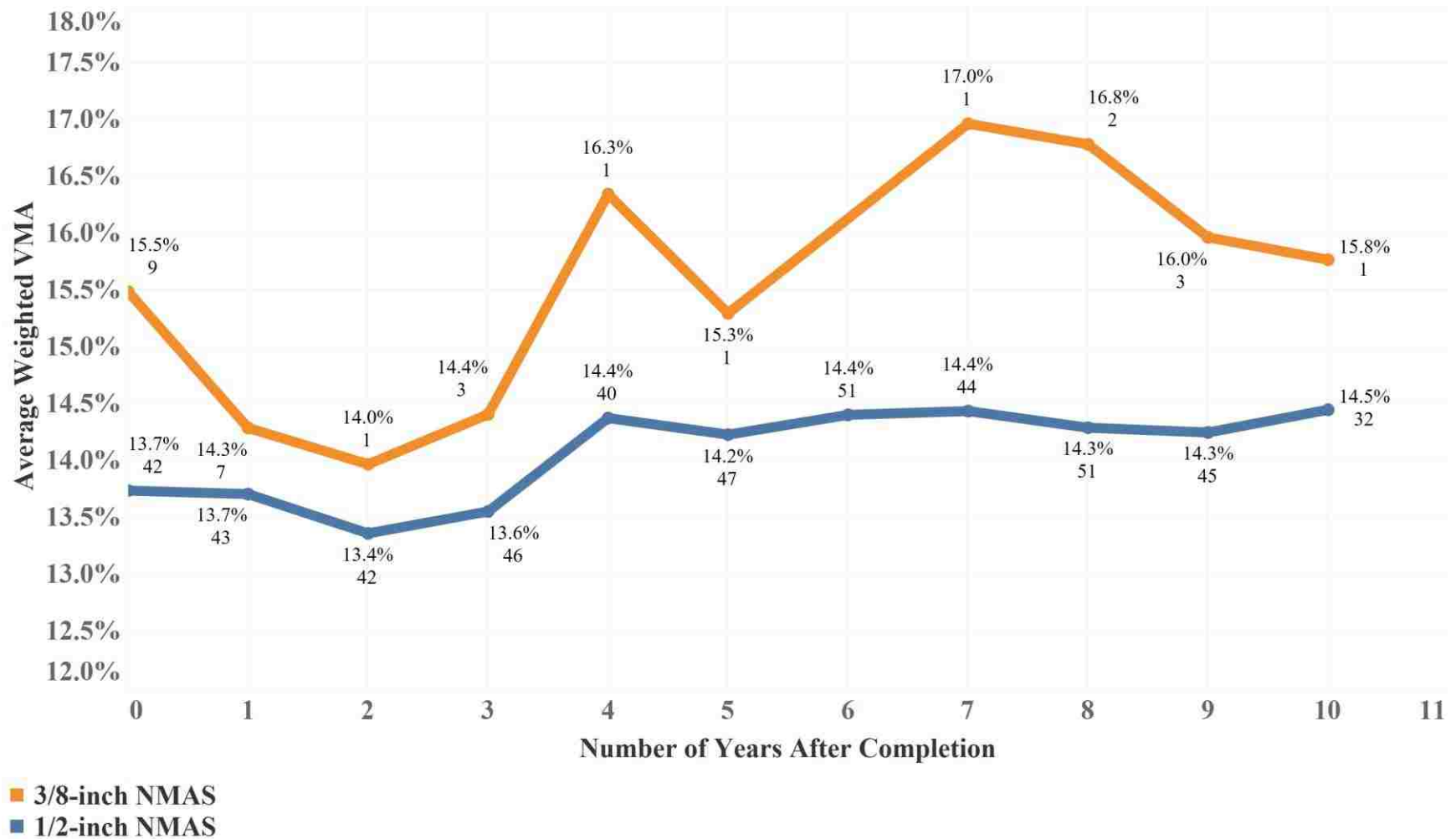
Figure 18. Average Weighted VMA Field Results by Tons of Mix and Number of Contracts Versus Number of Years After Contract Completion for 3/8-inch and 1/2-inch NMAWSDOT Asphalt Pavement Mixtures, 2007 to 2017 [Data Labels: VMA (Top), Number of Contracts (Bottom)]
