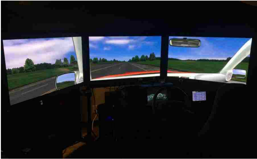
Figure 3.1 miniSim Fixed-Base Driving Simulator
