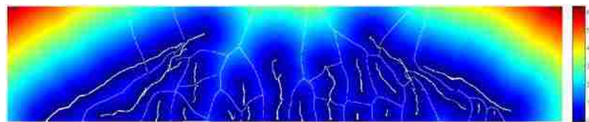
(c) The watershed regions and cracks.
