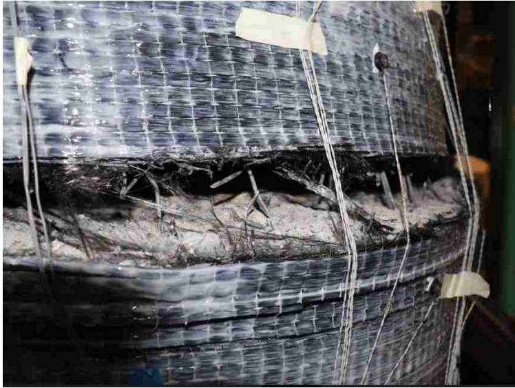
Figure 7-15. Widened fiber split on north face during Series 11
