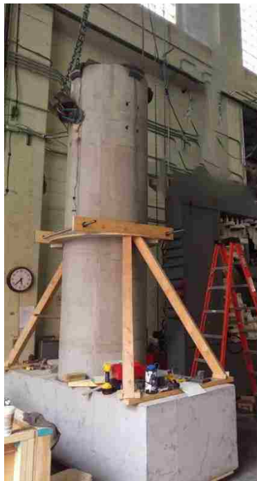
Figure 6-15. Pile-column braced on top of cap beam
