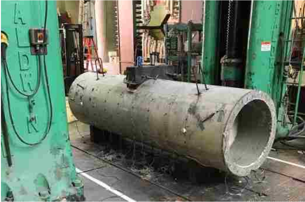
Figure 3-29. Three-point bending test optotrak and instrumentation
