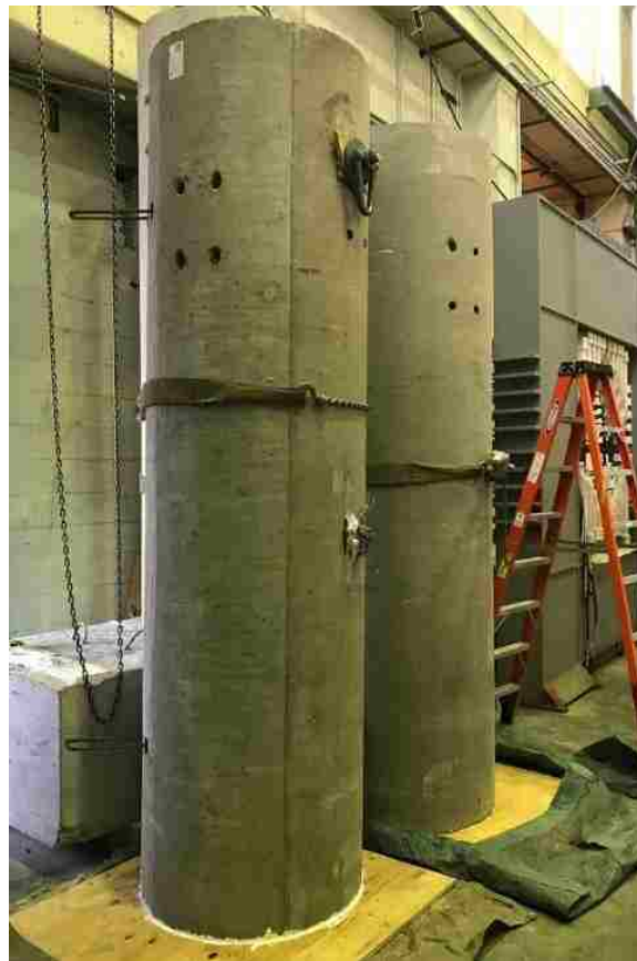
Figure 3-12. Specimen orientation prior to casting fill concrete
