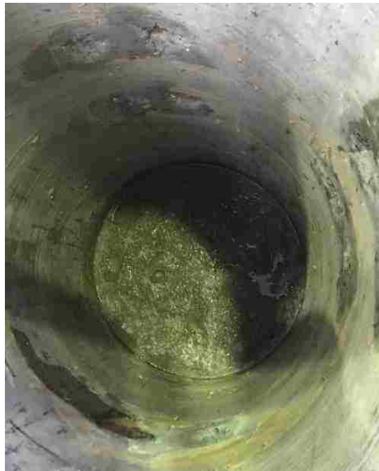
Figure 3-19. Middle diaphragm cast into Three-point bending specimen
