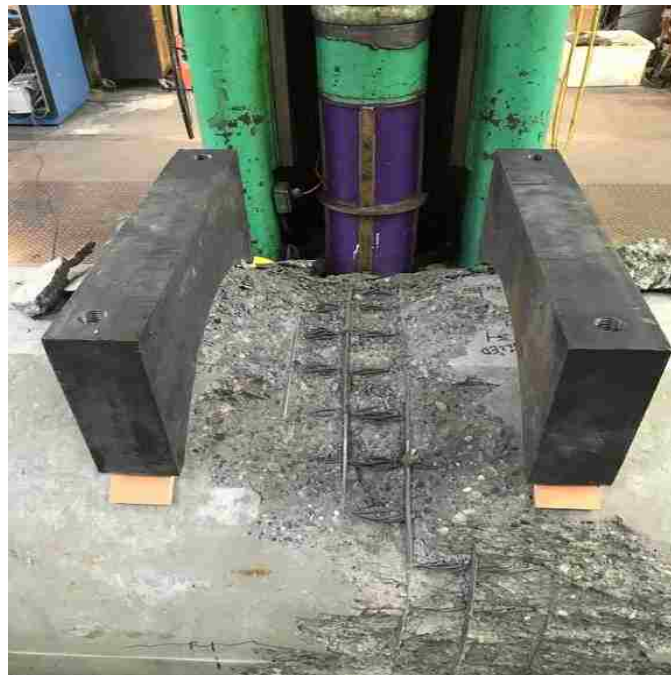
Figure 4-2. Concrete crushing and buckled strands
