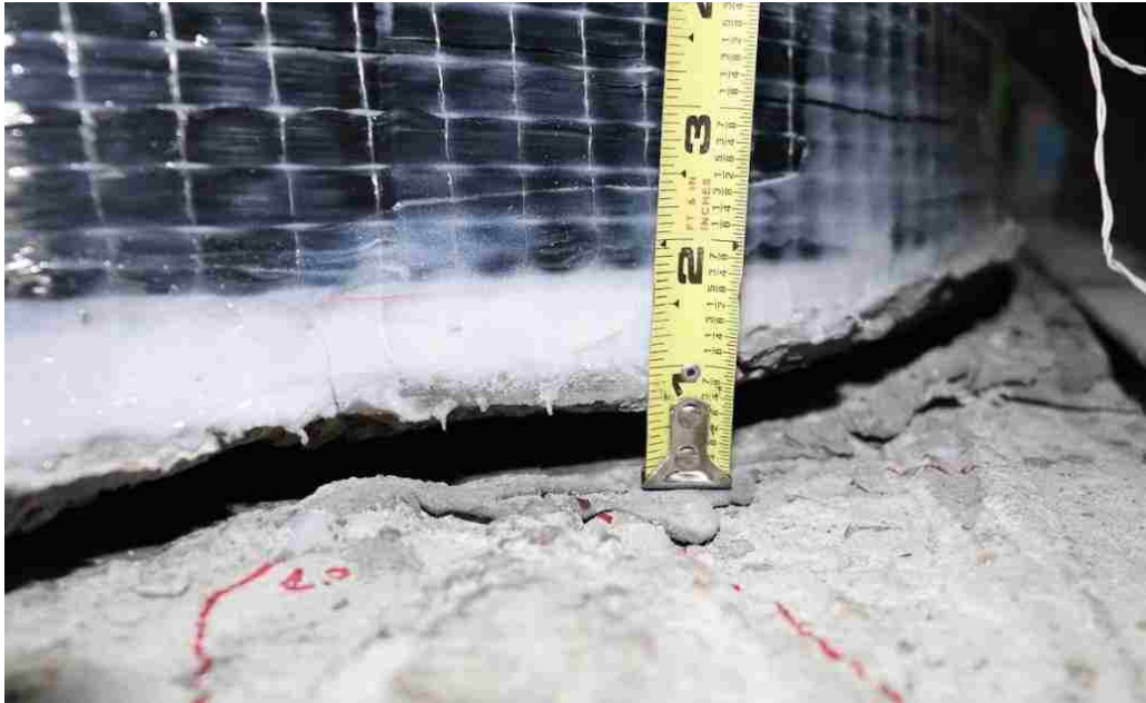
Figure 7-7. Uplift on Cycle 3 of Series 7 (+3.71%, -4.54% drift)
