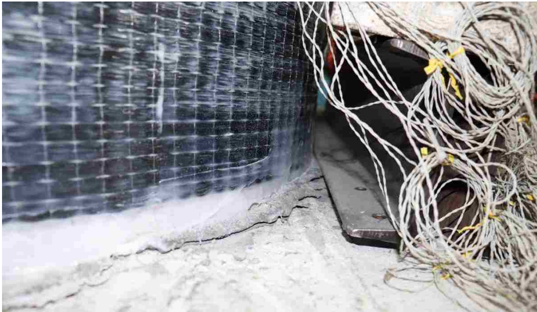
Figure 7-4. Uplift on Cycle 3 of Series 3 (+0.78%, -1.20% drift)
