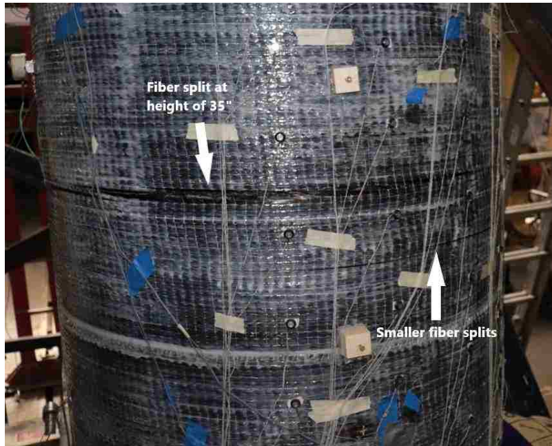
Figure 7-10. Fiber splitting on north face during Series 10
