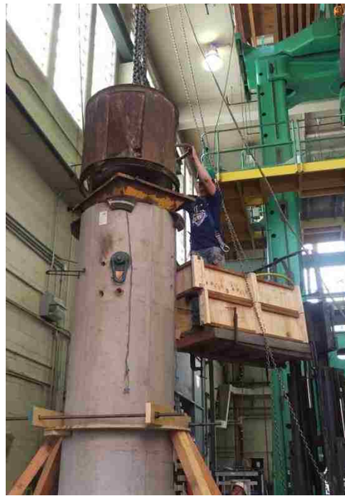
Figure 6-16. Casting plug inside of pile-column
