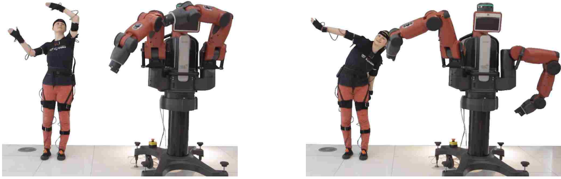
Figure 8.2: Remapping human motion to a robot model with different kinematic structures using interaction mesh. By continuously remapping human motion to robot model, we obtain a teleoperation method that works between agents with different kinematic structures.
