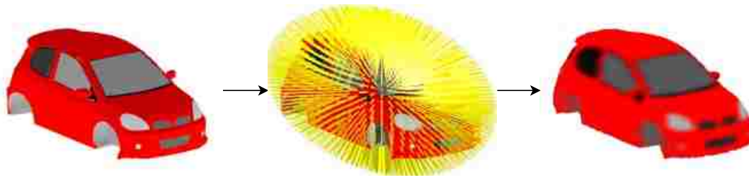
Figure 5.2: Processing meshes into hedgehog representation. On the left we have an input mesh, which is processed using a number of rays sufficient to capture a desired level of detail. On the right we have the hedgehog projection.
