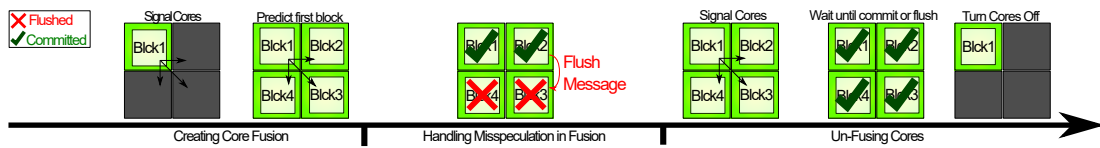
Figure 2.7: Core Composition Mechanisms for the EDGE-based architecture.
