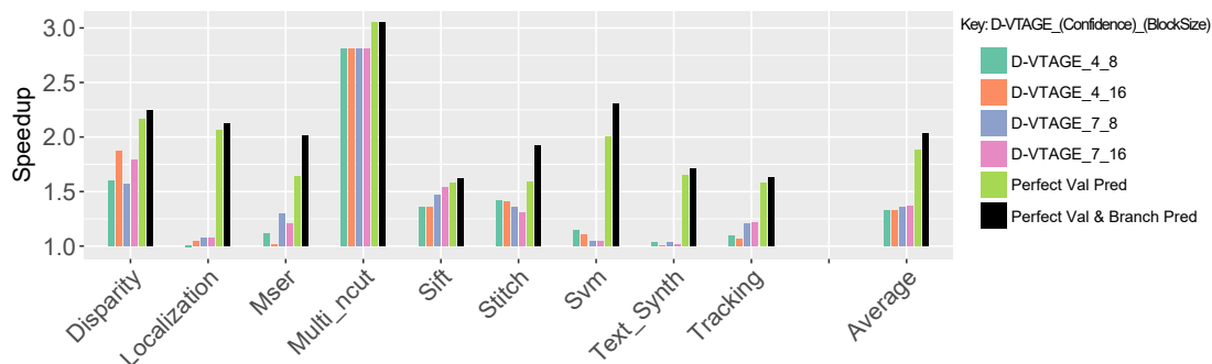
Figure 7.18: Speedup obtained using a D-VTAGE value predictor and RRF with 16 cores composed. Baseline is 16 cores composed with SF and without value prediction. Both use a non-perfect branch predictor. Higher is better.
