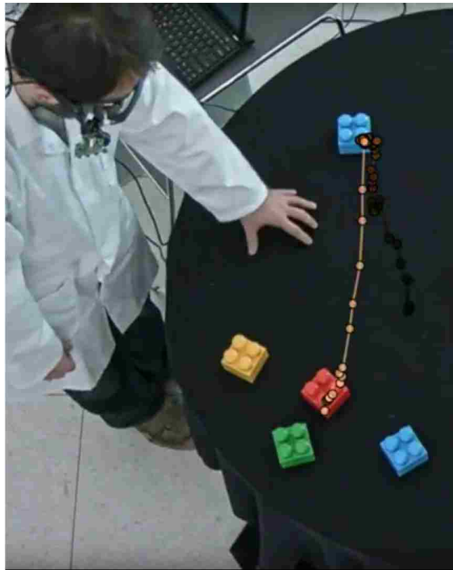
Figure 17: A short sequence of recorded 3D fixations from an experimental trial is projected into the ceiling camera frame of reference and overlaid on the captured image.
