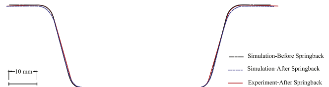
Fig. 13. Comparison of the obtained final shapes before and after spring-back from simulation with the final shapes after spring-back from experiment at wider opening end. The numerical result agrees well with the experimental data.
