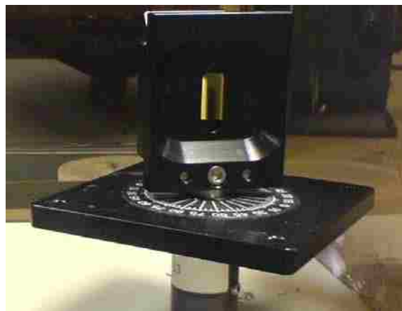
Figure 3.8: Graduated base rotatable solid sample holder.
