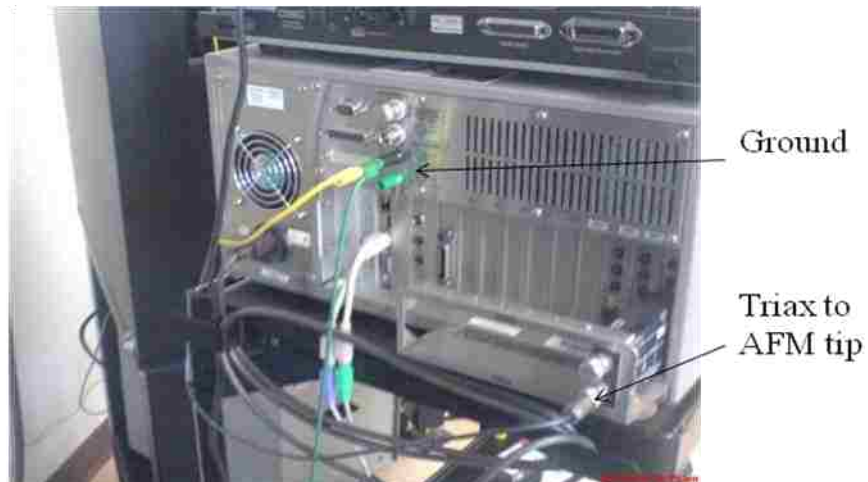
Figure 4.11: Circuit wiring of Keithley 4200-SCS.
