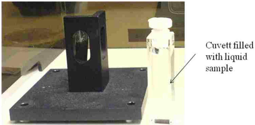
Figure 3.7: Liquid sample holder and a cuvette filled with liquid sample.
