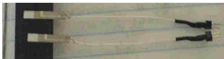
Figure 4.13: Ceramic probe substrate to isolate the AFM tip from the scanner circuitry.
