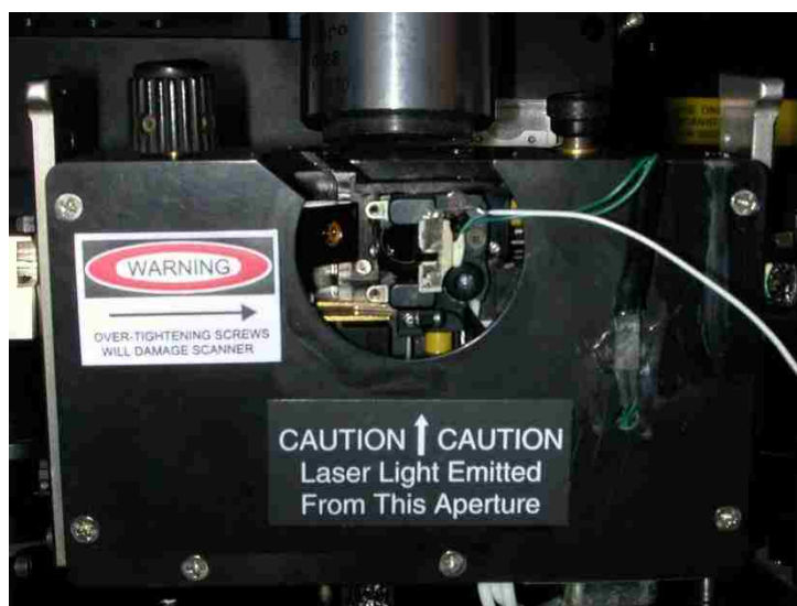
Figure 4.12: AFM scanner showing the tip mounting region.
