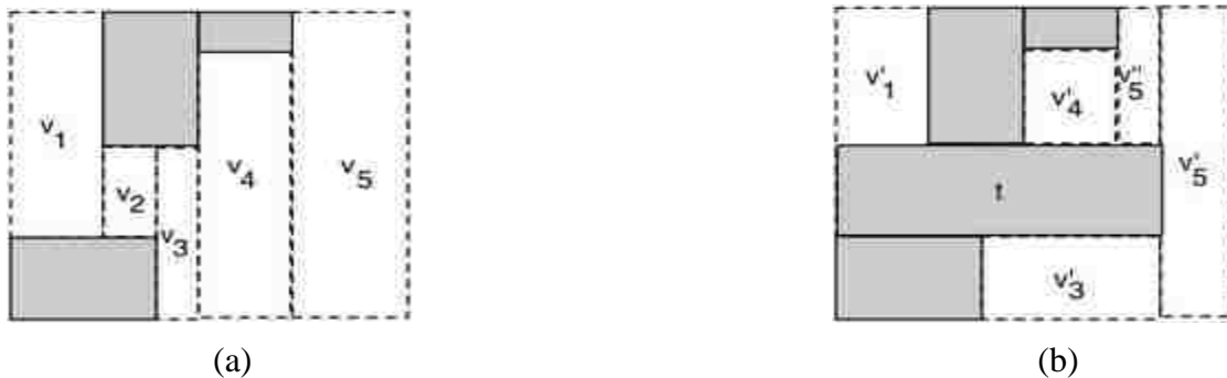
Figure 6-4 Placing a task in an MHS strip and updating MVSs accordingly: (a) before insertion and (b) after insertion
