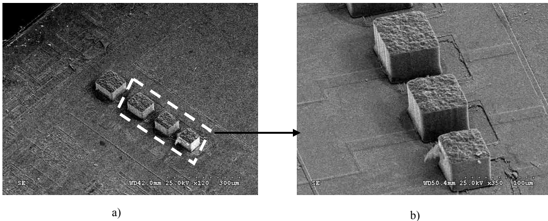
Figure 6.21: a) A probe array on a CMOS IC chip formed by pulse electroplating. b) A close view of the same probe array.
