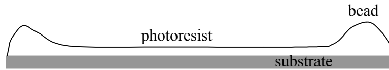
Figure 3.2: Edge bead usually shows up at the edge of the substrate when resist is thick. The bead profile is exaggerated in the above drawing.
