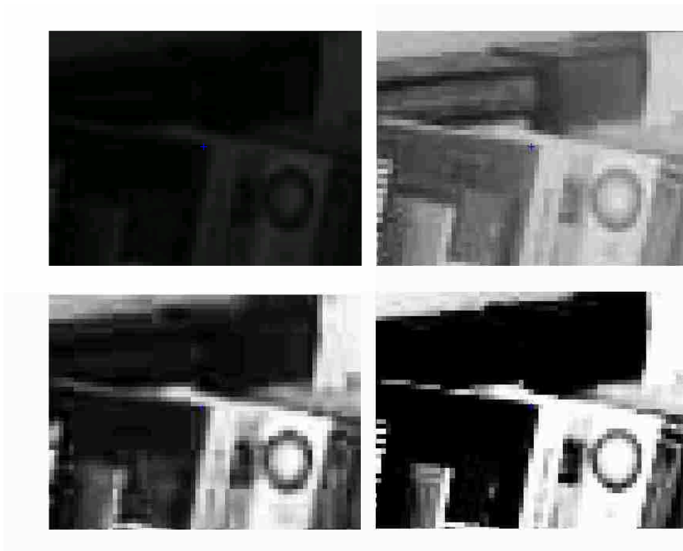
Fig. 17.: Upper row: Images at two different illumination conditions. The center pixels are marked. Lower row: Corresponding illumination normalized images based on the contrast signatures of the center pixels.
