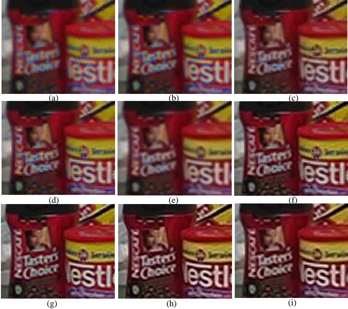
Fig. 40.: Demosaicking and super-resolution results. (a) Single frame demosaicking by bilinear interpolation. (b) Single frame demosaicking by edge directed interpolation [2]. (c) Single frame demosaicking by adaptive homogeneity directed interpolation [1]. (d) Proposed single frame demosaicking by all constraints applied, \sigma_I = 1.41, \sigma_S = 1.41, T_d = 5, T_o = 0, T_c = 2 , domain window is [5 \times 5] , iteration number is 3. (e) Multi-frame demosaicking, all constraints applied. Demosaicking is applied in 3 iterations, \sigma_I = 1.41, \sigma_S = 1.41, T_d = 5, T_o = 0, T_c = 2 , domain window is [5 \times 5] . (f) OSR result using single frame demosaicking in 3 iterations. (g) DSR without consistency set using single frame demosaicking in 3 iterations, T_d = 5, T_o = 0 . (h) DSR with all constraint sets applied in 3 iterations, \sigma_I = 1.41, \sigma_S = 1.41, T_d = 5, T_o = 0, T_c = 2 , domain window is [5 \times 5] . (i) DSR using multi frame demosaicking with all constraint sets applied in 3 iterations, \sigma_I = 1.41, \sigma_S = 1.41, T_d = 5, T_o = 0, T_c = 2 , domain window is [5 \times 5] . Iteration number for super resolution is kept 3 during the experiment.
