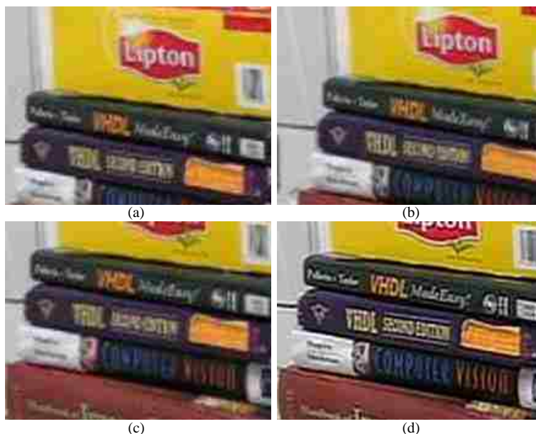
Fig. 4.: Spatial resolution enhancement of degraded images. 37 images are used in this experiment, 3 of which are shown in (a),(b),(c). SR image is given in (d).
