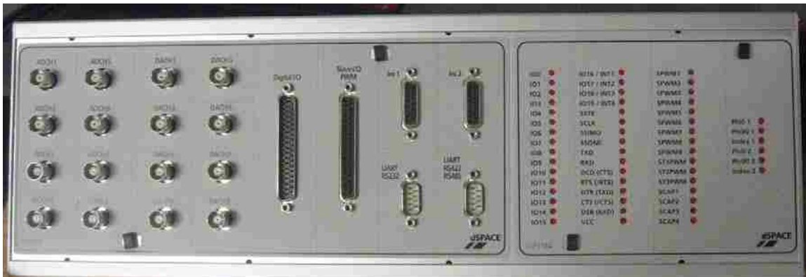
Figure 1.4 CP1104 I/O board
