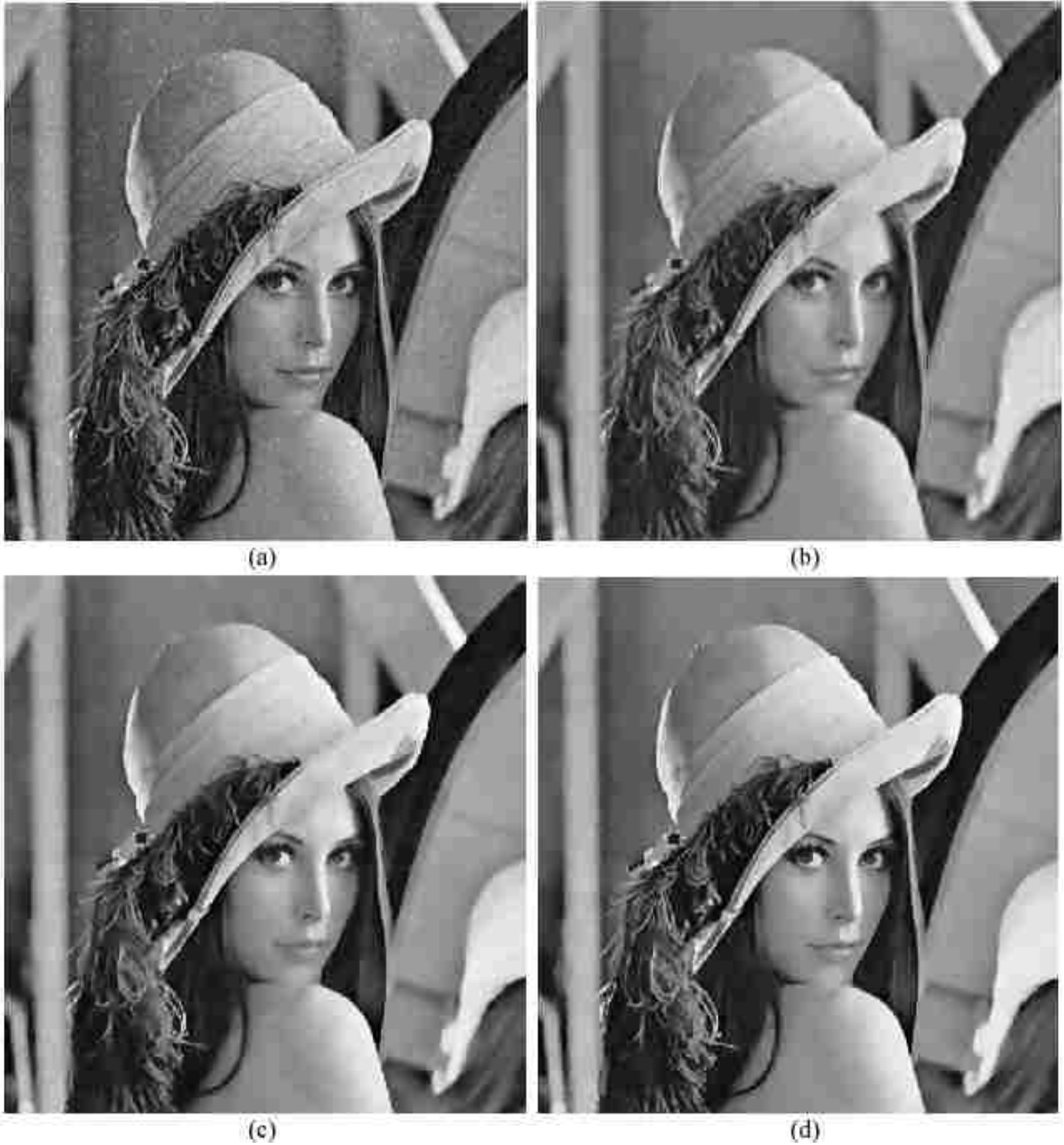
Figure 4.1 a) Input image with a PSNR 30.02, (b) The BayesShrink method[10], (c) The bilateral filter [1] with \sigma_d=1.8 and \sigma_r=5\sigma_n , (d)The proposed method with the number of decomposition levels is 1. For the proposed method, \sigma_d=1.8 and \sigma_r=3\sigma_n at each level. The wavelet filters are db8 in MATLAB.
