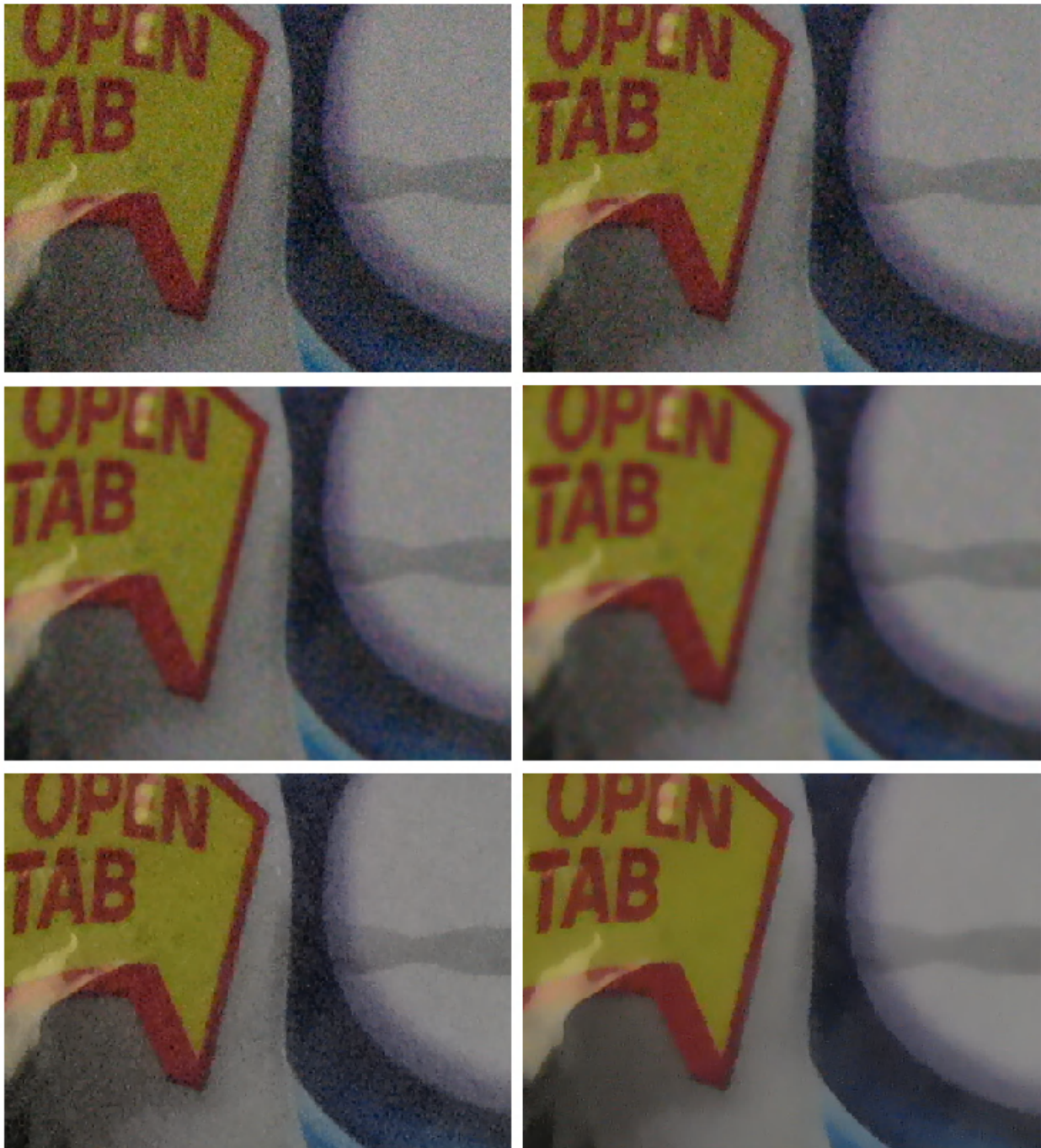
Figure 4.2 Real noisy image comparisons. (a) Input image, (b) The bilateral filter [1] with \sigma_d=1.8 and \sigma_r=3\sigma_n , (c) The bilateral filter with \sigma_d=1.8 and \sigma_r=20\sigma_n , (d) The bilateral filter with \sigma_d=5 and \sigma_r=20\sigma_n , (e) The proposed method with the decomposition levels is (1,4,4) for the (L,a,b) channels, respectively, (f) The proposed method with the decomposition levels (2,4,4). For the proposed method, \sigma_d=1.8 and \sigma_r=3\sigma_n at each level. The wavelet filters are DB8 in MATLAB.
