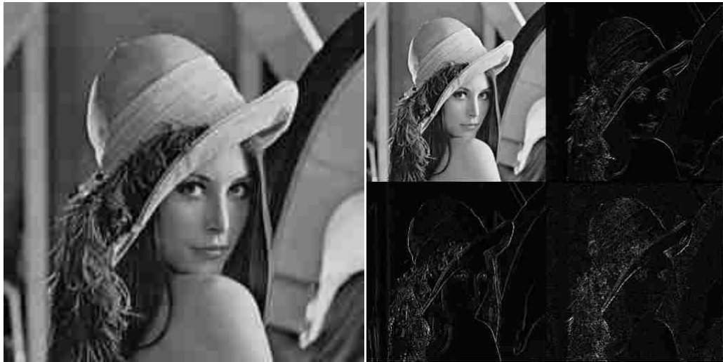
Figure 1.3 Right one shows the wavelet decomposition of the left picture. It uses 1 level Db4 wavelet decomposition in the Matlab. The image size is 512 \times 512
