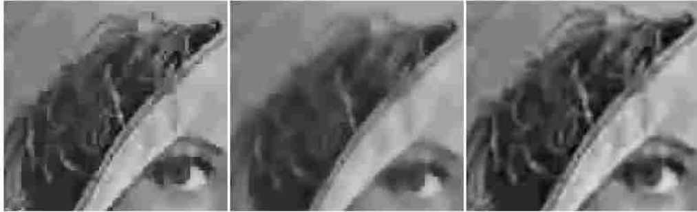
Figure 6.5 Performance of Bilateral Filter. From left to the right: input compressed image, bilateral filtered image and adaptive bilateral filtered image.
