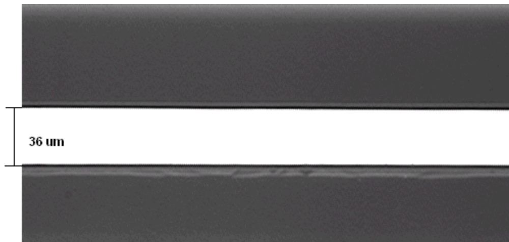
Figure 28 Pentacene channel window on silicon wafer.
