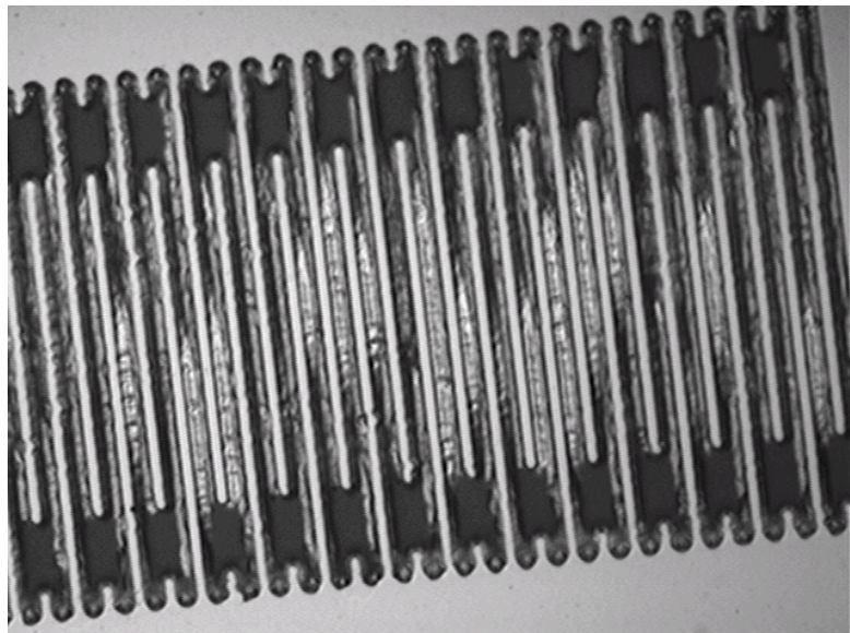
Figure 14 Schematics of chlorobenzene lift-off IDT result.
