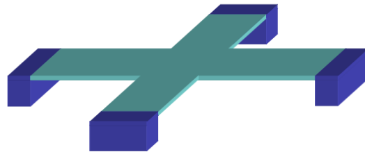
Figure 2.2 A schematic figure of the practical stage which is stiff in all horizontal directions. A second, perpendicular beam is added.
