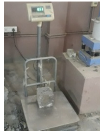
Figure 4. Weight loss test on concrete cube.
