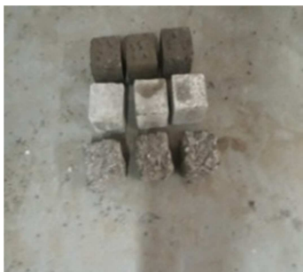
Figure 3. Cubes after chemical attack.
