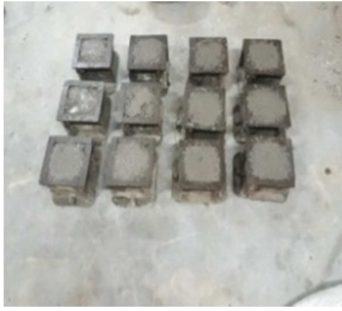
Figure 1. Casting of cube specimens.
