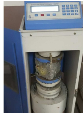
Figure 5. Compression test on cube.
