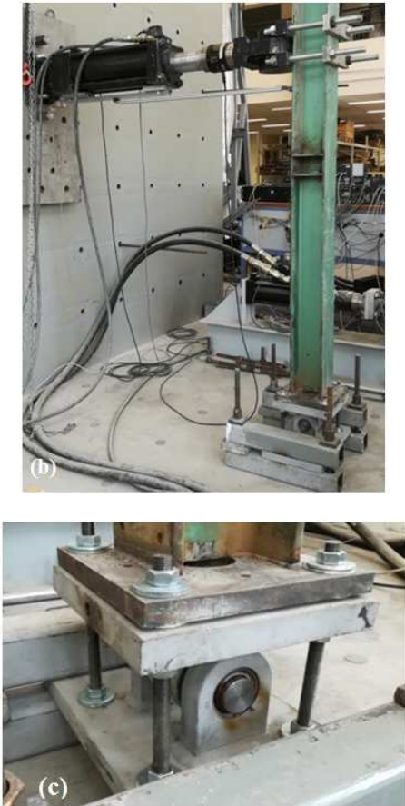
Figure 6. (a), (b) Test setup, (c) clevis connection.
