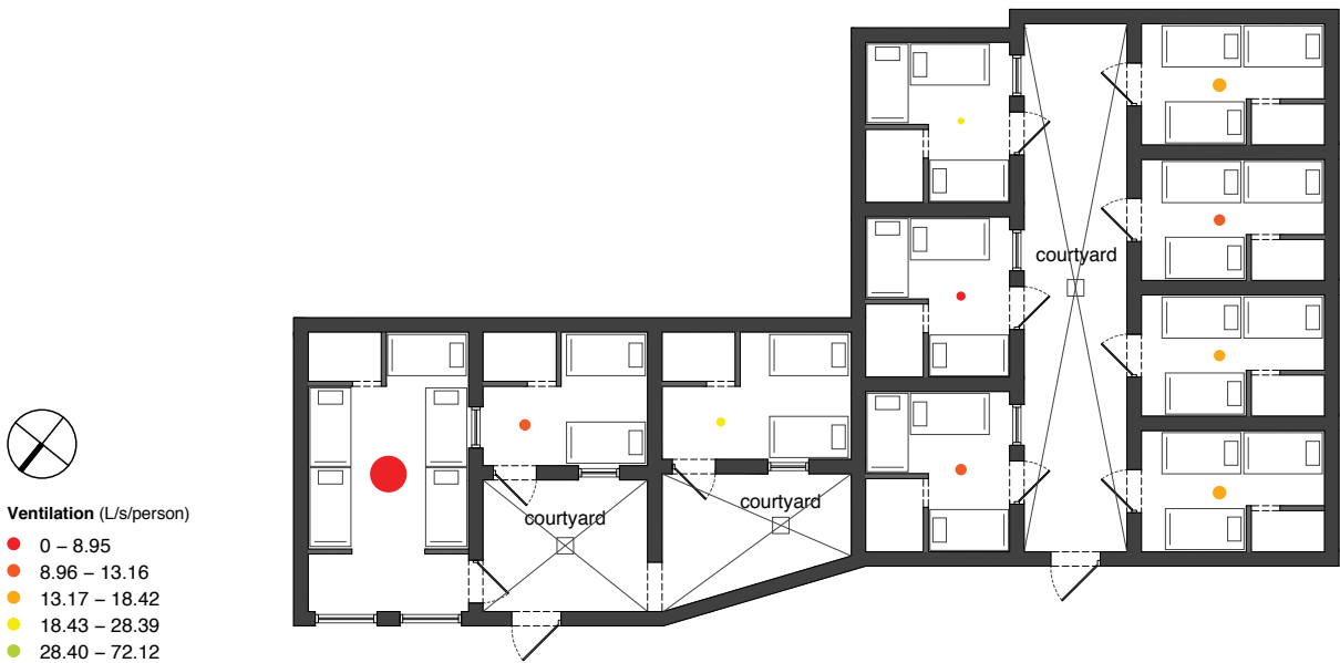
Figure 6. Architectural floor plan of UPRB with overlay of per person ventilation (colored dots). Colored dots are proportional to the number of inmates per cell.
