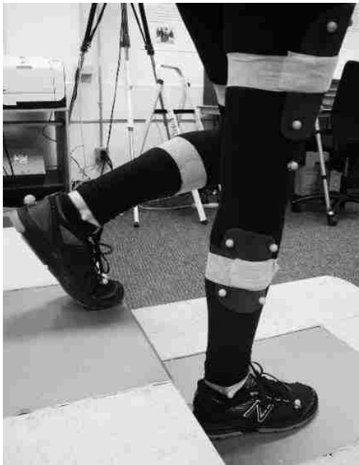
Figure 9. Platform setup with force plates imbedded and a model demonstrating the step task. Note the reflective marker placement. Image by Kim M. Poulsen.
