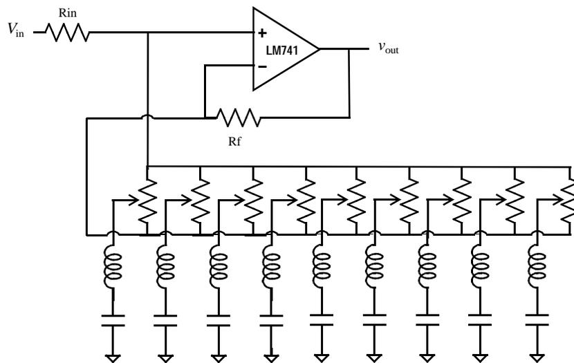
Figure 2 — Graphic equalizer circuit.
