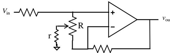
Figure 3 — Simplified Graphic equalizer circuit.
