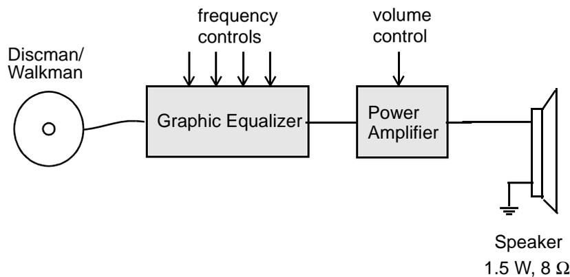
Figure 1 — 3-band audio graphic equalizer block diagram.
