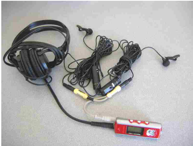
Figure 9. Fully assembled recording kit: recorder, splitter, two lapel microphones and headphones.
