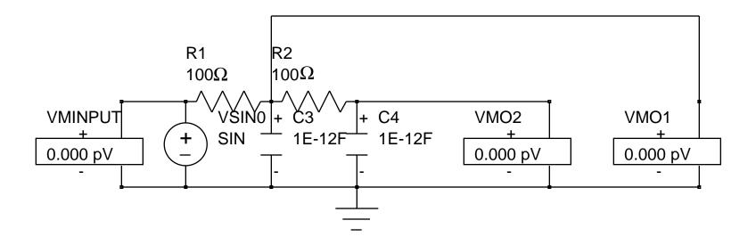
• An ac analysis can be used to generate frequency domain plots of magnitude and phase of the transfer function
