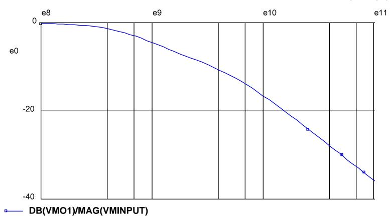
• Note that the frequency is in Hertz in SPICE, so it must be scaled by  $2\pi$  for comparison with our Bode plot
