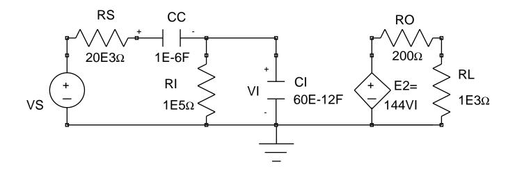
• This capacitor adds a zero (at zero frequency) to the transfer function which we can observe from a SPICE simulation, or calculate and Bode plot
