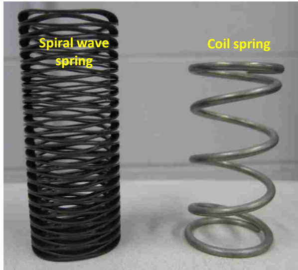
Figure 4.15. Custom designed crest-to-crest spiral wave and conventional coil springs
