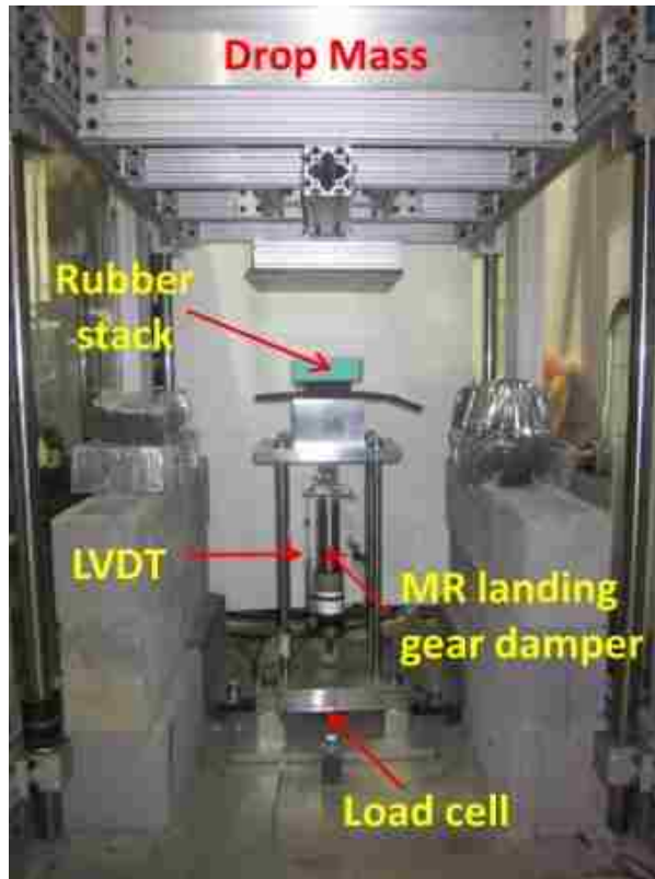
Figure 5.1. Single MR landing gear damper drop test setup at the University of Maryland MR: magnetorheological
