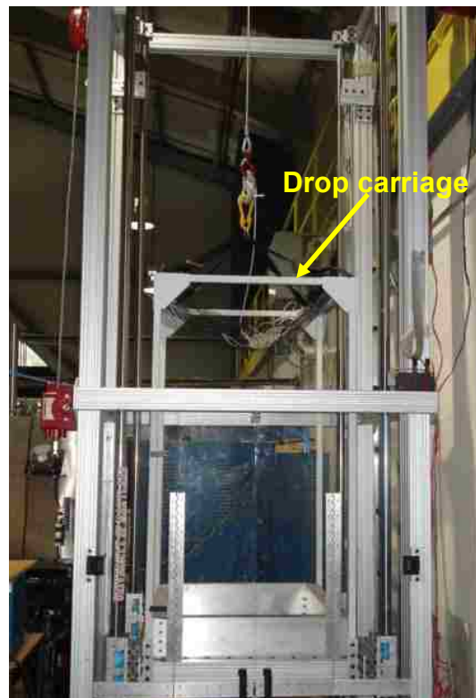
Figure 2.10. Drop test carriage at the University of Maryland College Park
