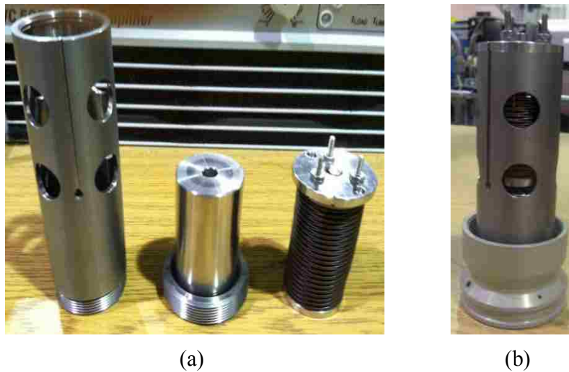
Figure 4.22. Spiral wave spring-based passive relief valve with a dummy bobbin; (a) components of the spiral wave spring-based relief valve and (b) Valve assembly
