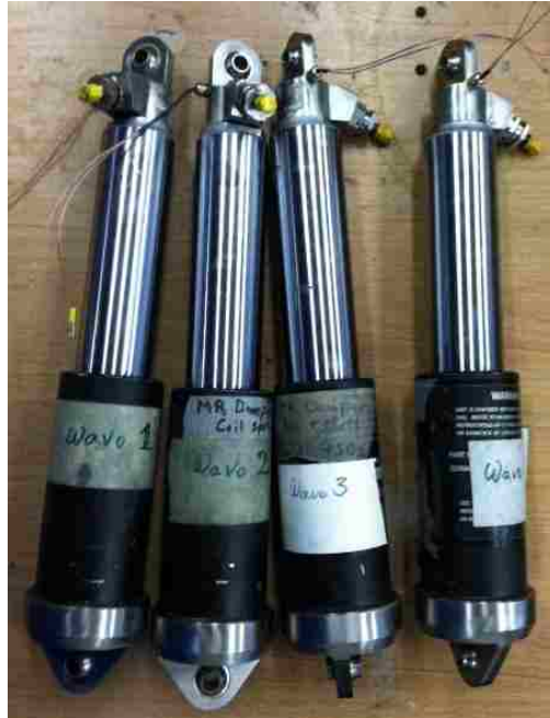
Figure 5.9. Photograph of the four spiral wave spring-based MR landing gear dampers used for the iron-bird drop test
