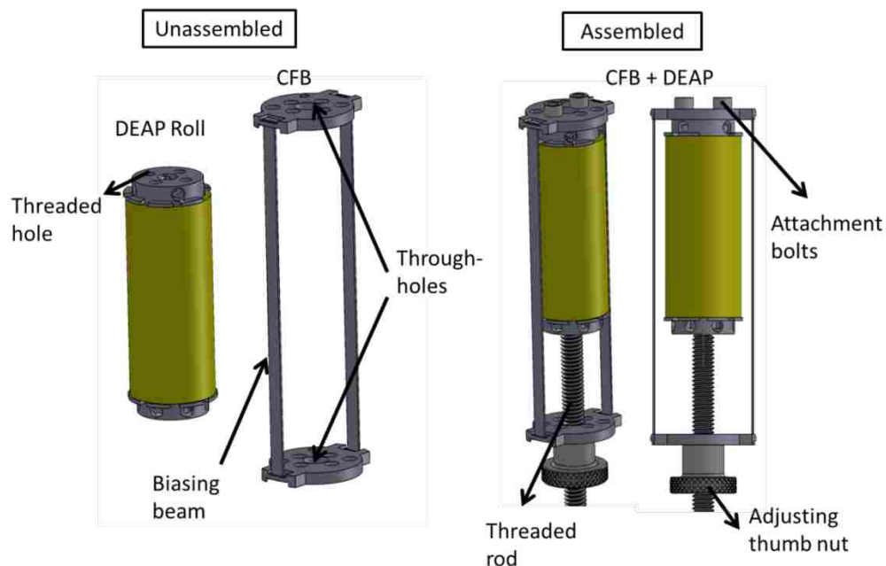
Figure 5.2 CAD drawing of CFB actuator prototype. CFB element and DEAP roll unassembled view (left). Assembled CFB actuator (right).
