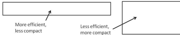
FIGURE 3.6: Wing aspect ratio trade-off: efficiency and compactness
