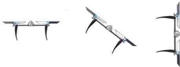
FIGURE 2.3: Equilibrium transition from hover to forward flight
