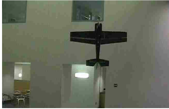
FIGURE 1.10: Fixed-wing MAV capable of hover, [24]
