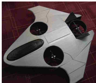
FIGURE 1.15: Fan-in-wing configuration MAV
