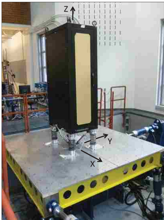
(a) Cabinet installed on 6 DOF hydraulic shaker table.
