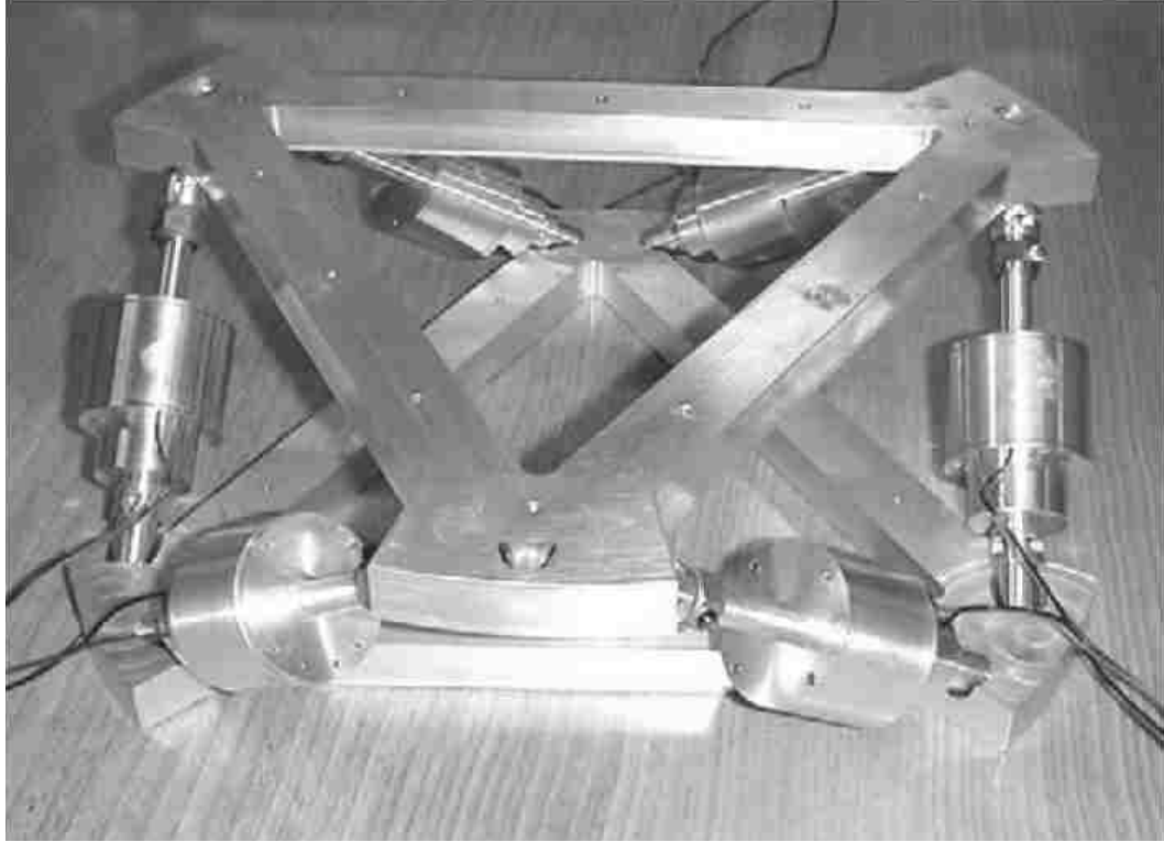
Figure 1.14: Cubic hexapod manipulator with piezoelectric actuators [36].
