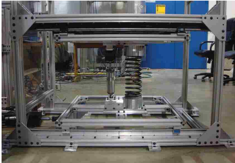
Figure 5.9: Lateral 1-DOF shake table test stand.
