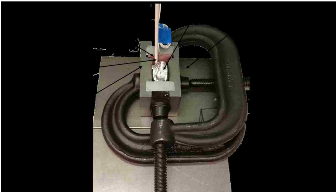
Figure 2.1. Casting setup used for aluminum casting.
