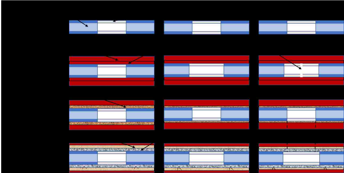
Figure 8. Schematic of the mechanism of the sensor at 350°C and 600°C for different fiber-copper interface.
