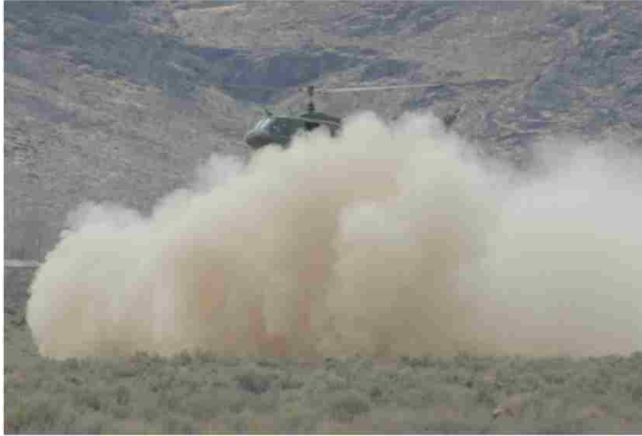
Figure 1.1: A helicopter encountering brownout conditions during a landing in the desert. (Photo courtesy of Optical Air Data Systems LLC).
