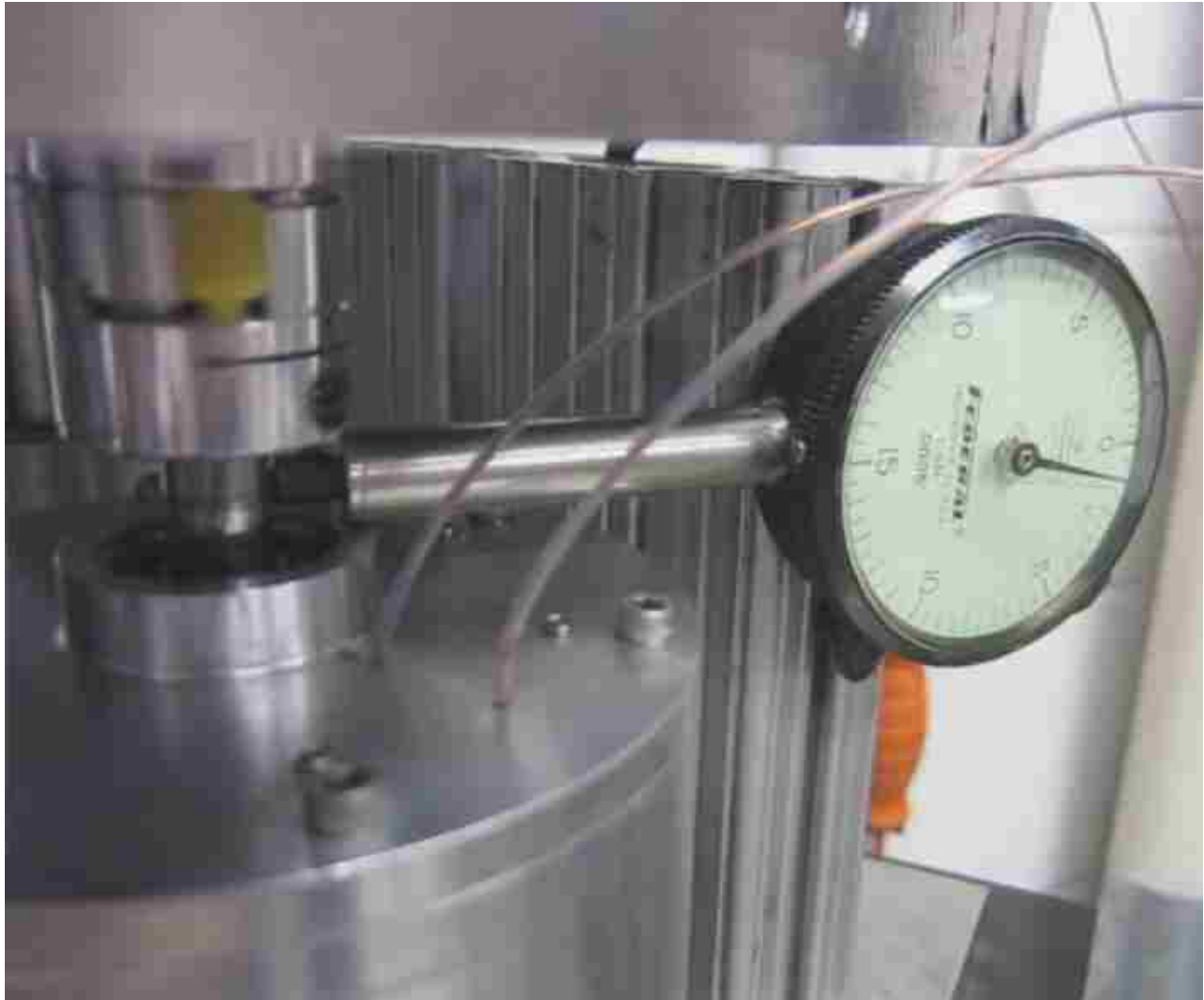
Figure 5.11 – Precision dial indicator used to measure the eccentricity of the rotating bob
