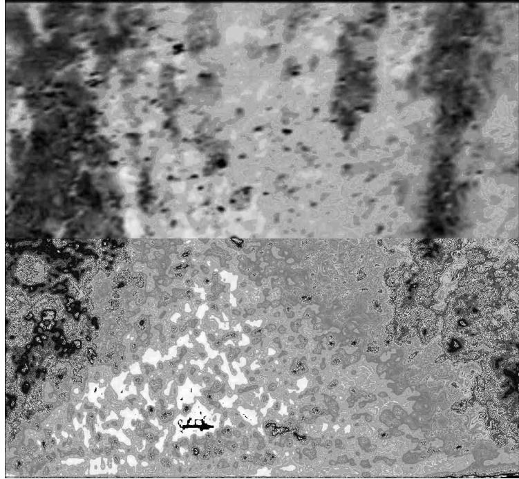
Figure 5.3 - Micrograph of robust column ends in squeeze-strengthened MR fluid, adapted from (Tao, 2001).
